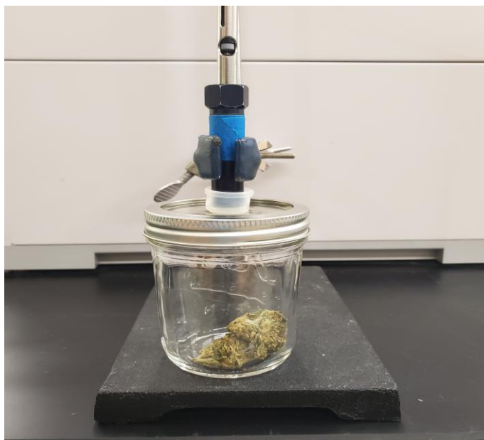
Figure 49. HS-SPME sampling process for hemp and marijuana.
