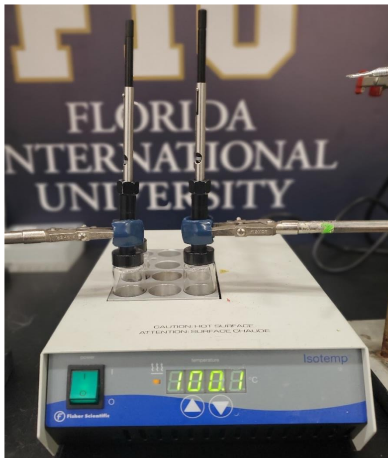
Figure 75. TPPO extraction setup using a heating block.
