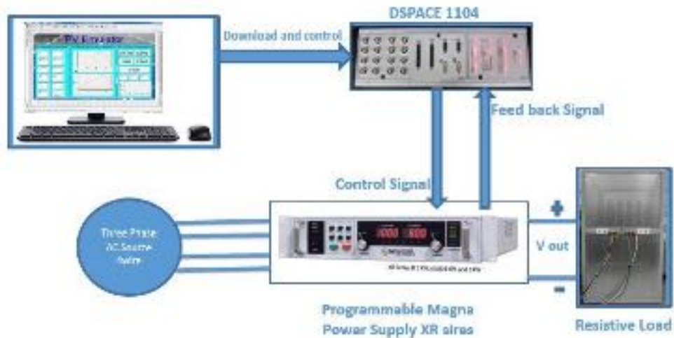
Figure 4-2 The PV emulator setup in our hardware testbed
