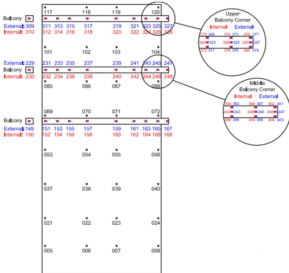
Figure 21 – Model Scale 1:25 – Pressure Tap Layout Side B
