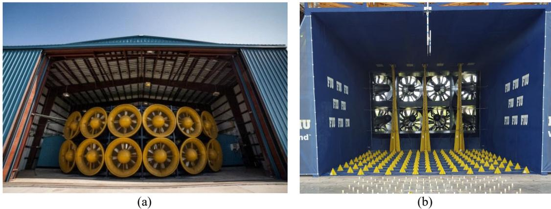
Figure 1 - (a) NHERI Wall of Wind Experimental Facility (WOW EF), FIU; (b) Spires and floor roughness elements
