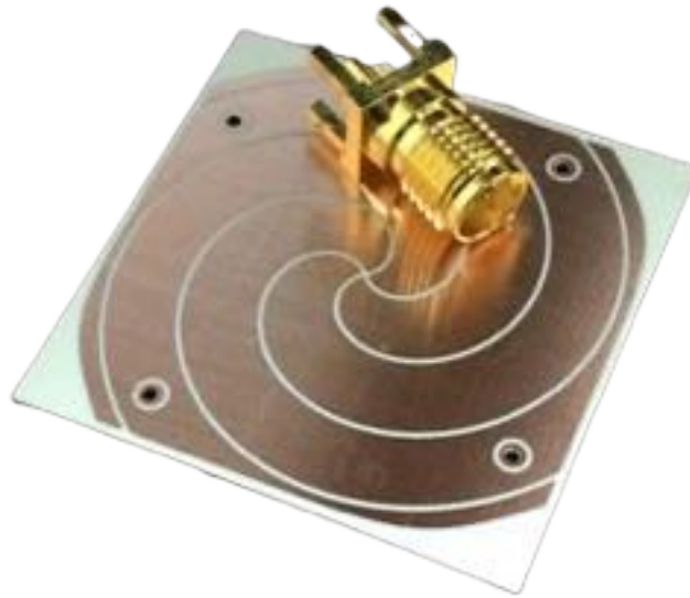
Figure 7 Symmetric, balanced fed antennas exhibit the self-cancellation property. Examples include cross dipoles, orthogonally fed patches, and four-arm spirals.
