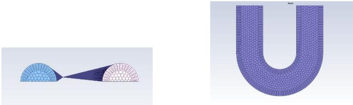
Figure 31: Polyhedral Mesh of Fluid for fine refinement test case with prism layers on Fluid-Pipe-Interface
