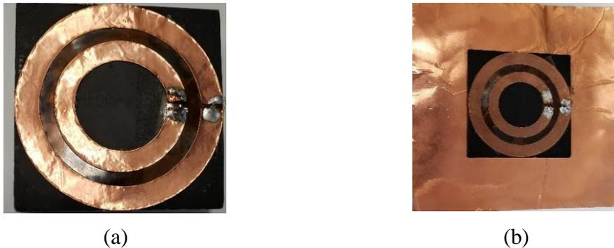
Figure 3.4. Fabricated CSCMR (a) with ferrite substrates in air, (b) with ferrite substrates over a metallic surface.
