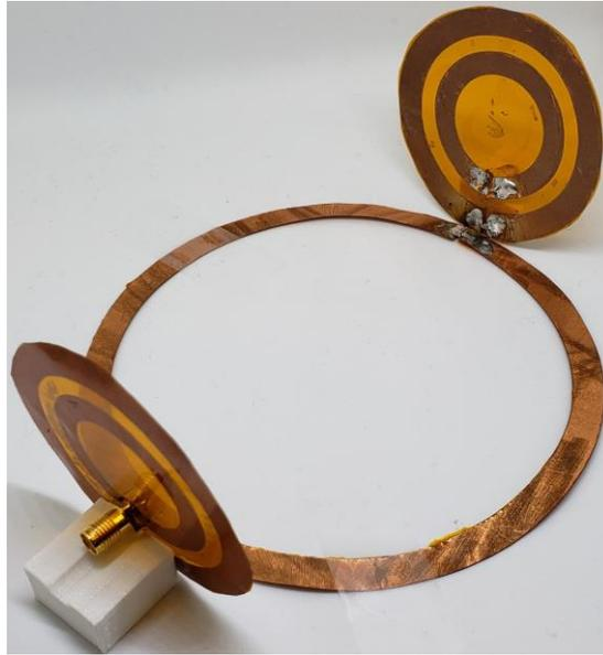
Figure 4.3. Prototype of the proposed CSCMR system with a simplified U-loop.
