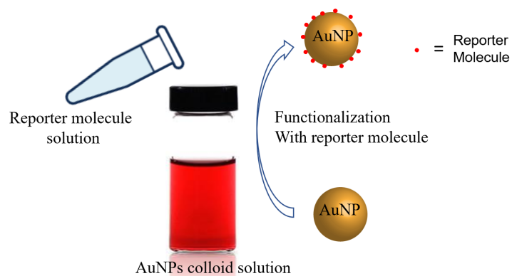
Figure 2-18 Schematic drawing of molecule modification of AuNPs colloid.
