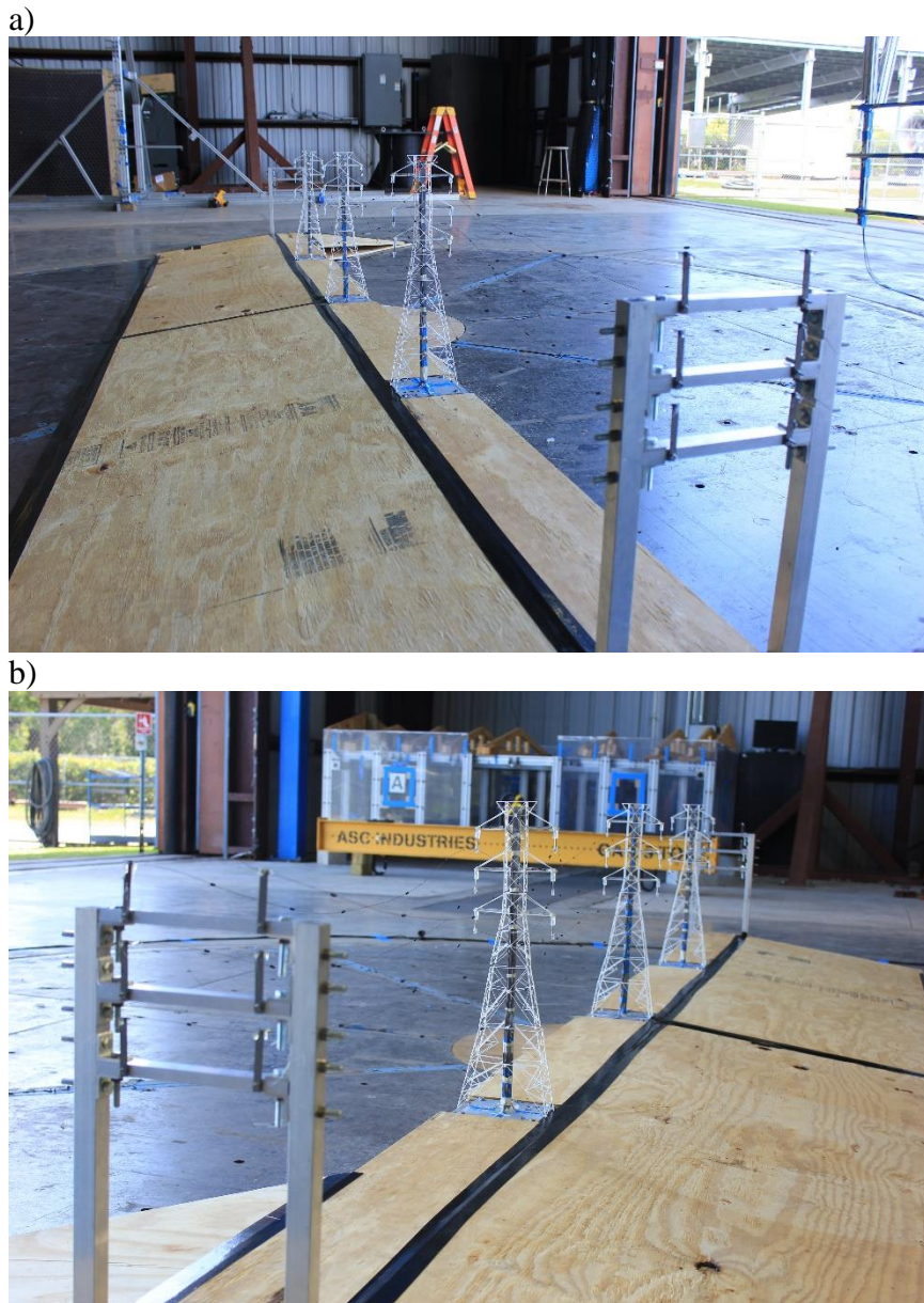
Fig. 3.4: Entire transmission line system: a) before testing, and b) after testing
