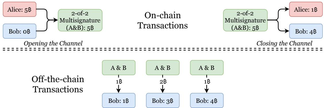
Figure 3.1: Off-chain payment mechanism between two Blockchain nodes
