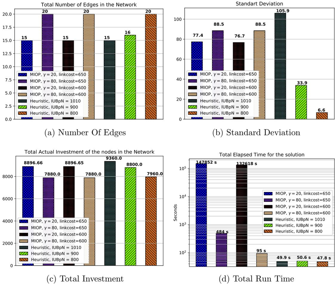
Figure 5.4: Heuristic approach compared to MIOP solution
