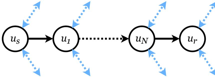
Figure 7.1: For a typical example the sender  $u_s$  initiates a transaction to  $u_r$  through the intermediary nodes  $u_{1..N}$ . A node can open as many channels as she wishes. The channels are assumed to be bidirectional.
