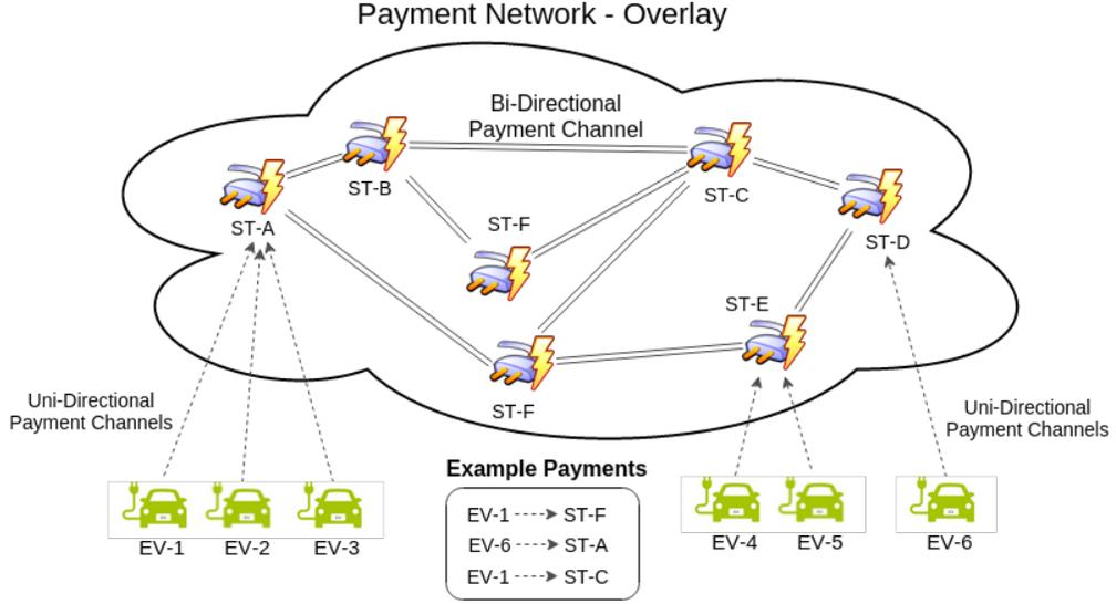
Figure 4.1: An overview of the envisioned Payment Channel Network (PCN) for the EV charging example.
