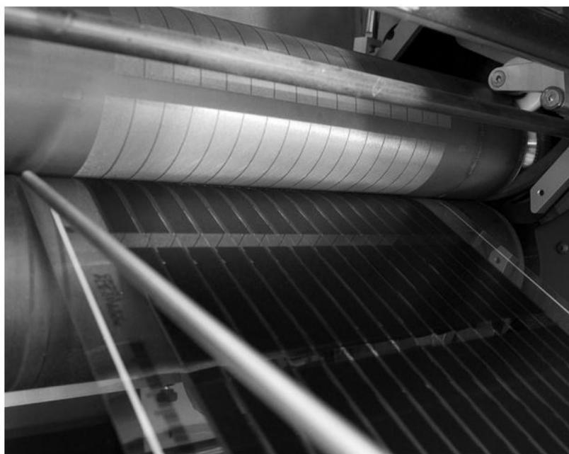
Figure 4.6: Illustration of a rotary screen printing of PEDOT. Reproduced from [70] with permission from Elsevier.
