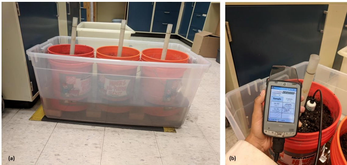
Figure 3-15. Photographic record of (a) laboratory set-up of all three lysimeters and (b) reading the surficial di-electric of the lysimeters using a Stevens Hydra Probe.
