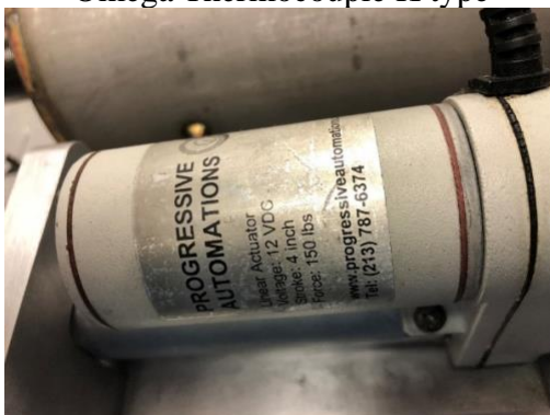
Progressive Automations Linear Actuator (force: 150 lbs.)
