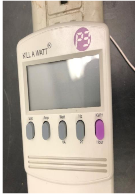
P4400 Wattmeter (max power 1800W)
