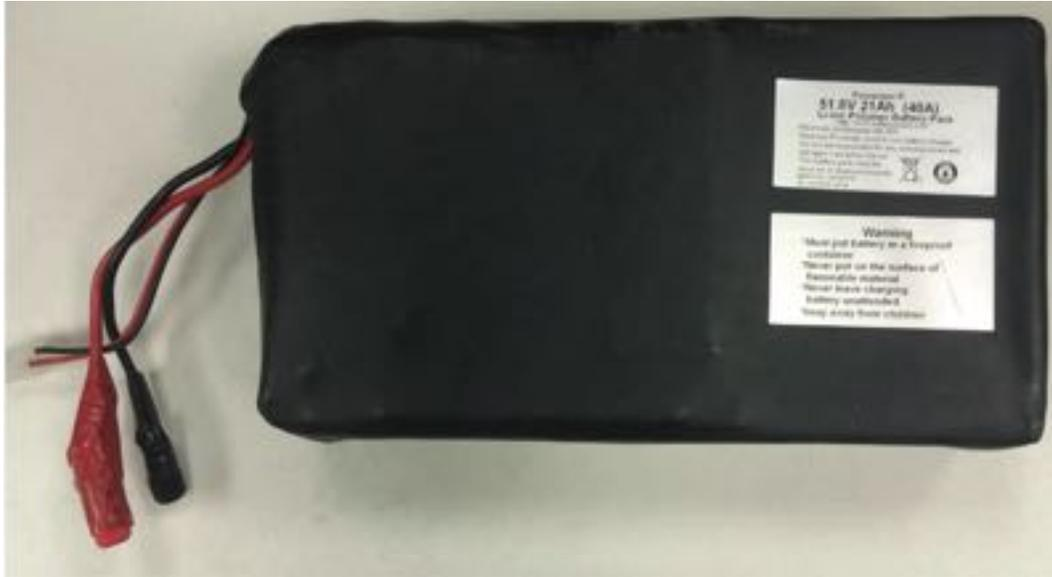
Figure 10.7 Lithium-ion battery bank module.
