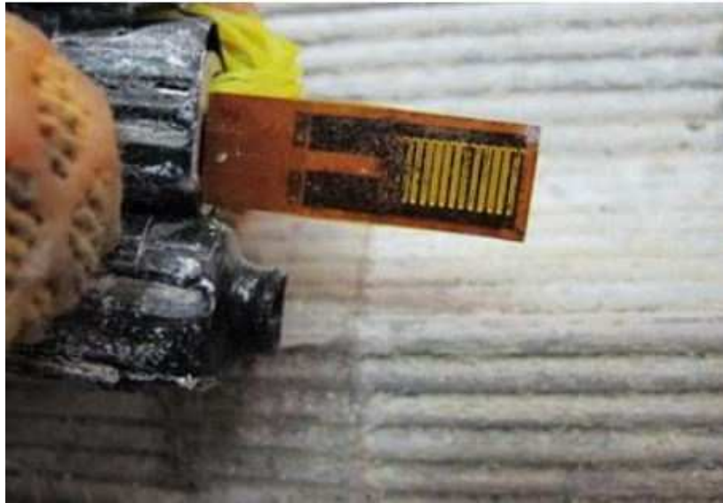
Figure 2-26: Close-up view of good LPR sensors after dissection [27]
