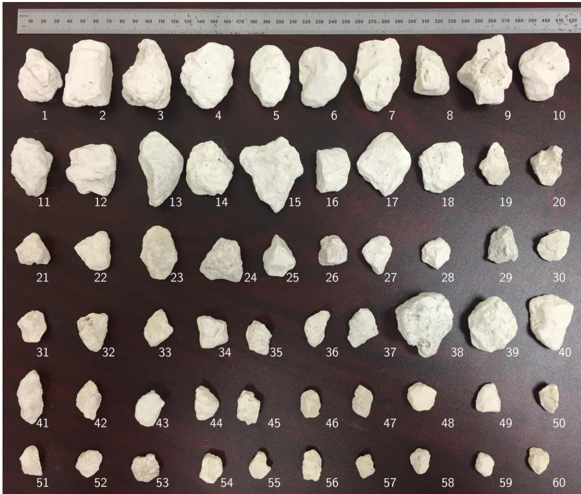
Figure 4.1. 60 particles used in SL scanning.
