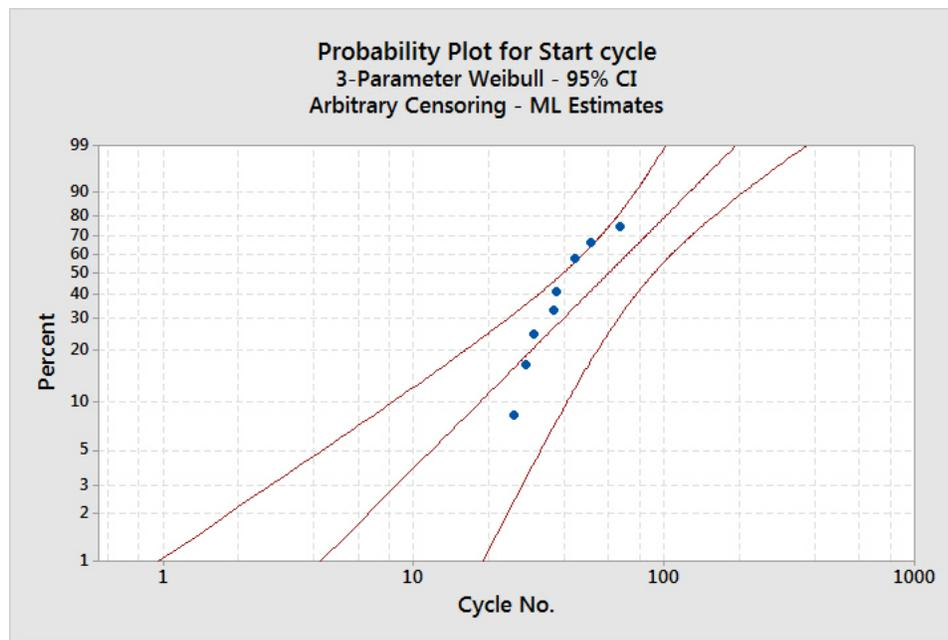
Figure 6.7: Weibull plot fit with the life cycle data for cyclic life tests of SLA battery
