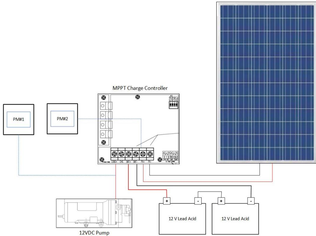
Figure 5.3: Electrical System Unit
