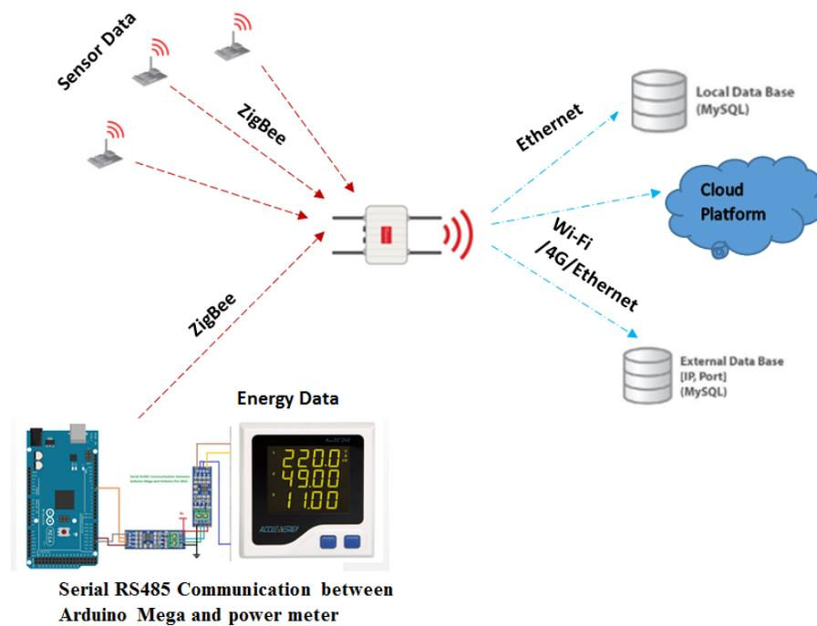
Figure 5.8: Data transmission, reception and storage scheme of the system
