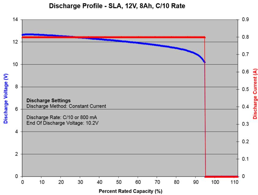
(a) Discharging profile of SLA battery
