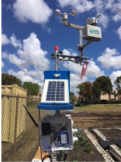
Figure 5.4: WSU connected to a weather station
