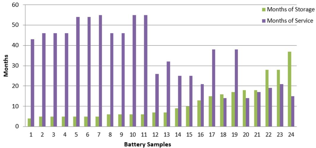
Figure 6.3: SLA battery service span against storage time
