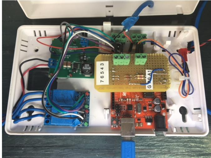
Figure 5.7: The control unit for scheduling irrigation events
