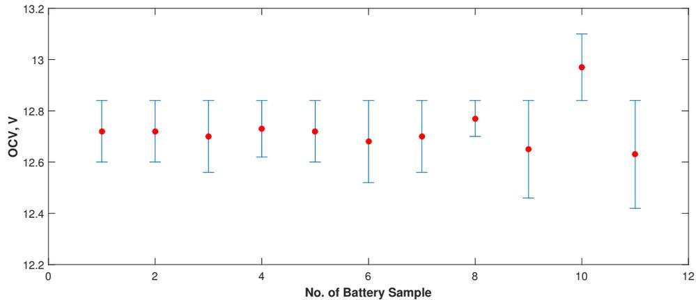
Figure 6.2: Measured OCV of new batteries
