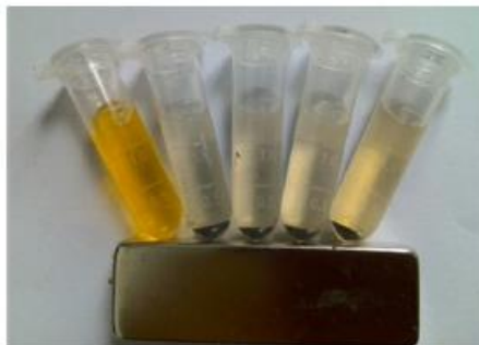
Figure 2.6 Decolorization of orange G with MGO-GOx-CPO in pure buffer and in actual wastewater with same amount of orange G added (From left to right, orange G in pure buffer without treatment, and orange G in water samples from Hei river, Fengyu, Qinzhen and a man-made lake after treatment).
