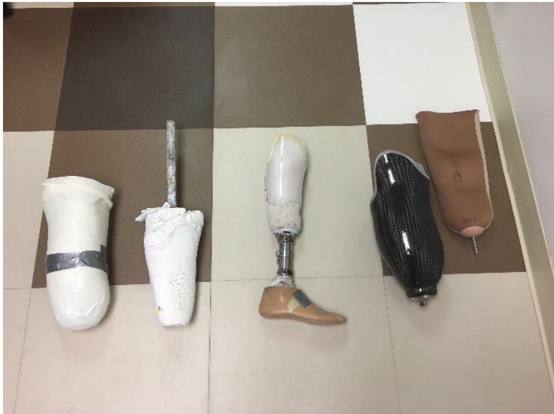
Figure 1. Prosthetic fitting process. from left to right the parts are the molding, filled mold, clear test socket, final fiber carbon socket, and the liner.
