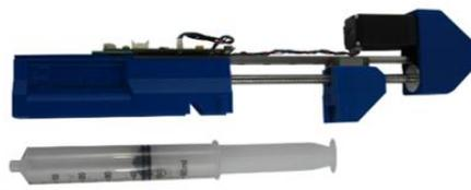
**Figure 58:** Print head syringe for low viscosity polymers respectively
