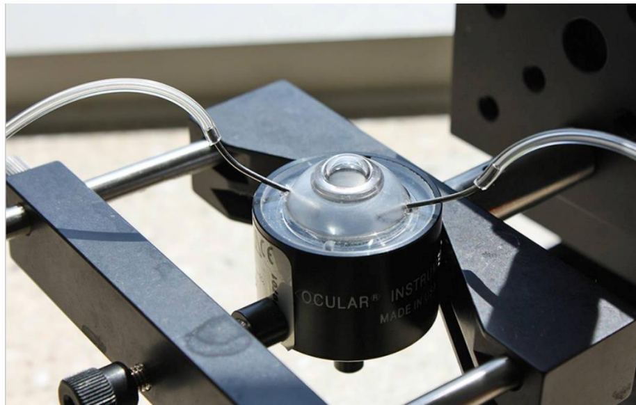
Figure 13.6 Optical phantom from Malik et al. 277 The custom-built ocular model. Glucose concentration in the anterior section is varied through the two infusion tubes.
