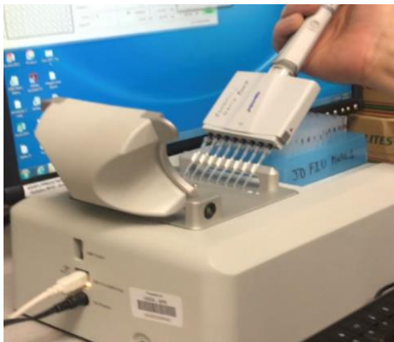
Figure 21: Nanodrop spectrophotometer: used to quantify nucleic acids in preparation for qPCR
