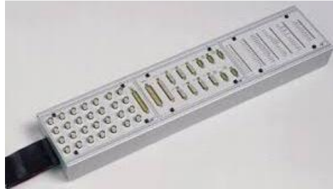
Figure 2.4 dSpace system for developing embedded controller
