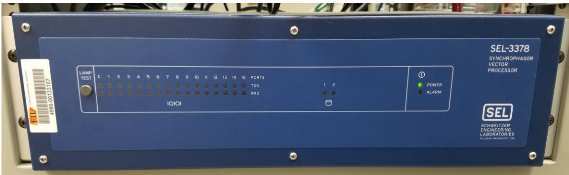
Figure 2.9 The Phasor Data Concentrator.
