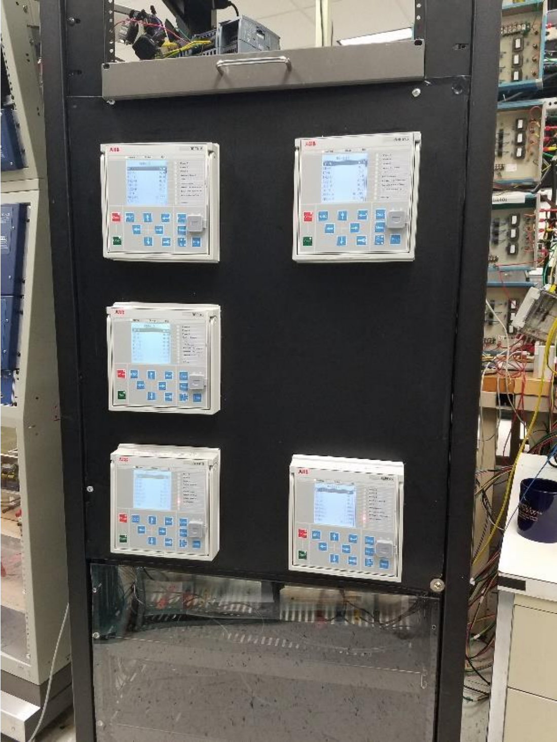
Figure 2.11 ABB IEDs Hardware Setup.
