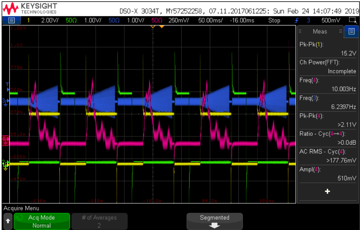
Figure 4.9. Oscilloscope image of CIT MS timing signals and mass spectrum
