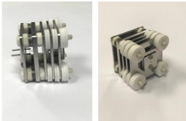
Figure 3.4. SS CIT integrated with test bed electron gun assembly
