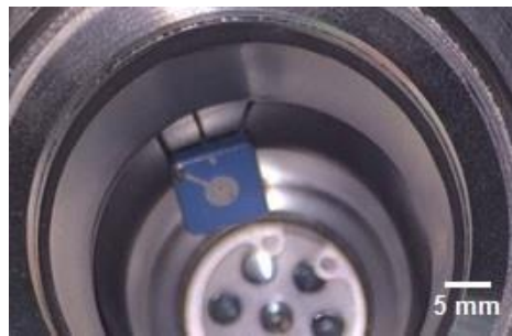
Fig. 3.16. CIT chip mounted in HV test chamber
