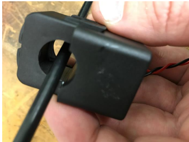
Figure 4.15. Clamp on toroidal transformer power measurement circuit
