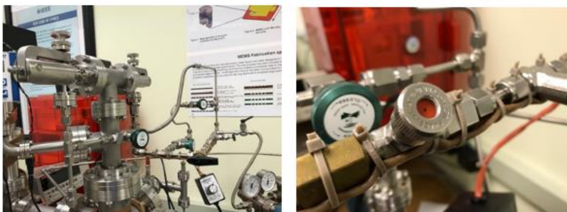
Figure 4.7. CIT instrument test bed analyte injection system and septum injection port
