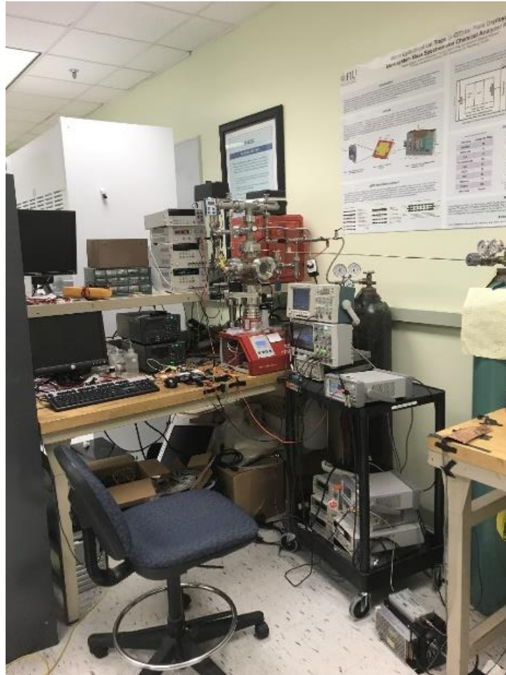
Figure 4.4. CIT miniature mass spectrometer test bed – chamber & electronics
