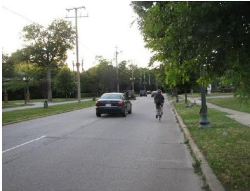
**Figure 2-6: Wide Curb Lane (Source: Mead et al., 2014)
