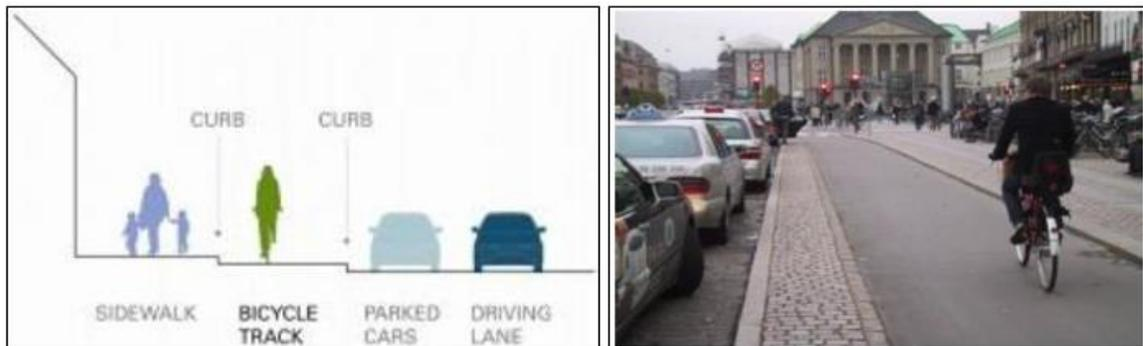
**Figure 2-4: Bicycle Track (Source: Mead et al., 2014)
