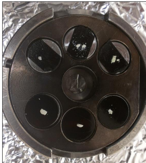
Figure 1. Precipitates loaded on studs using carbon tape and mounted for SEM
