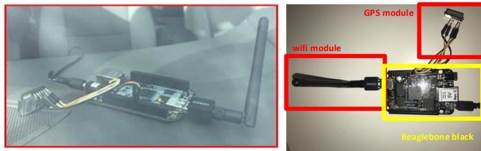
Figure 4.8 Testing module board interfaced with commercial GPS module.
