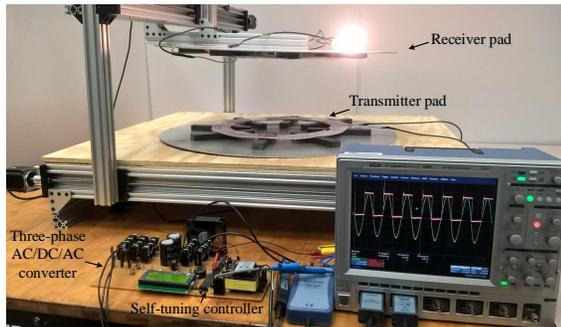
Figure 4.15: The IPT system setup comprised of primary and secondary pads, primary AC-AC matrix converter controlled using the proposed power transfer controller, and the secondary converter.
