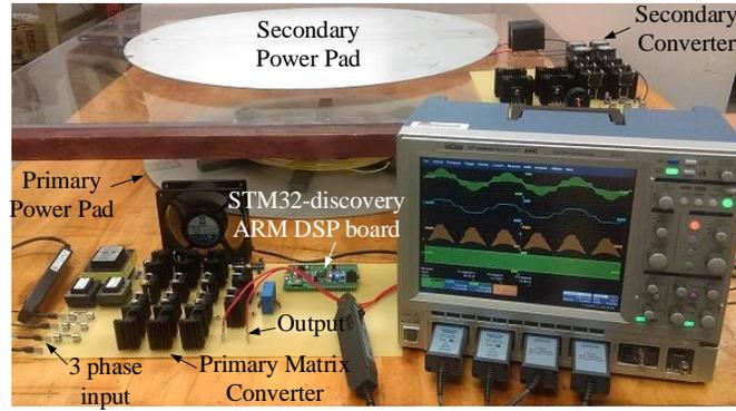
Figure 5.8: The case study IPT system with circular power pads.
