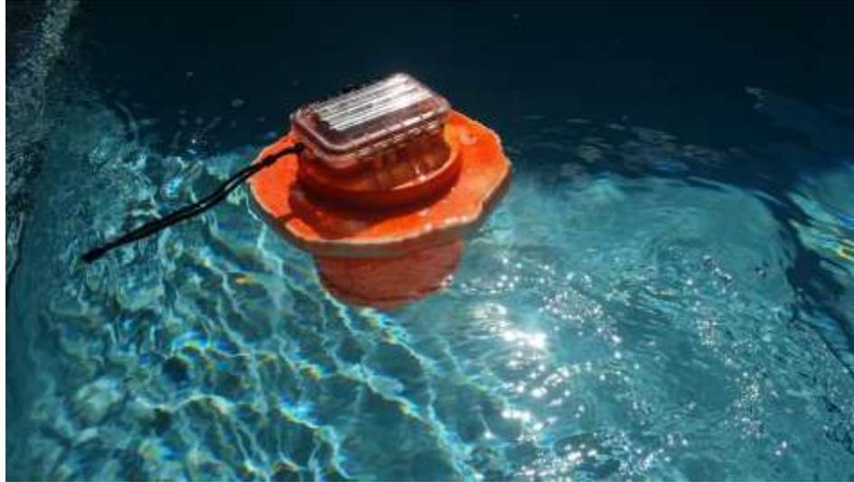
5-3. The GPS drifter is constructed out of a PVC body with a Garmin E Trek H GPS attached on top.
