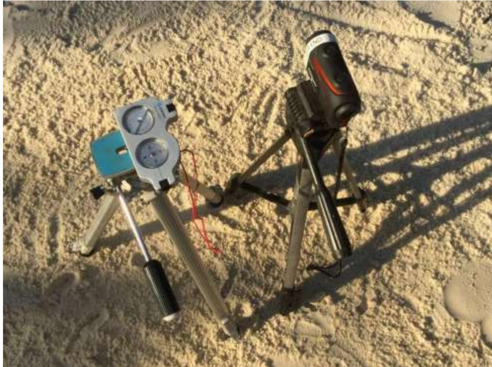
4-1. The Nikon Prostaff 7 Laser Rangefinder and Steren Electronics compass are mounted on a photographic tripod to measure the speed and path of a rip current. The speed is measured by calculating the distance with the laser rangefinder of a floating object moving inside the rip current over time. The compass is used to determine the angle of the rip path in order to correct the distance measurements for a non-linear rip current path.
