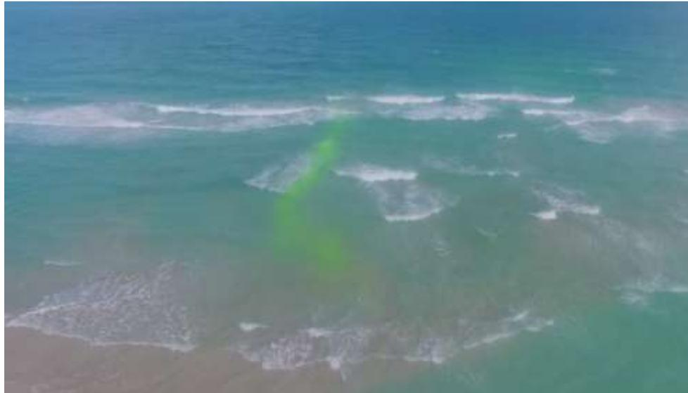
4-4. A weak rip current is delineated by fluorescein tracer dye and imaged by a DJI Phantom 3 Advanced Quadcopter at South Beach on January 12, 2017. This South Florida rip current shows a relatively straight path.
