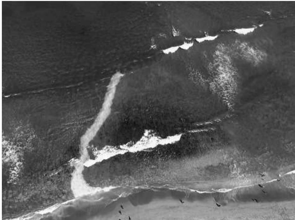
6-12. A freeze-frame from the quadcopter video of fluorescent dye at Ocean Reef Park, Palm Beach County shows that the rip current is fairly linear and terminates at the surf zone on April 27, 2016.
