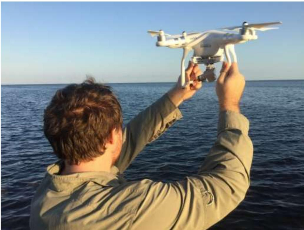
Figure 4-2. The DJI Phantom 3 Advanced Quadcopter is being prepared for takeoff. This drone provides an aerial view of rip currents delineated by tracer dye, allowing for analysis of the rip path with implications for escape methods.
