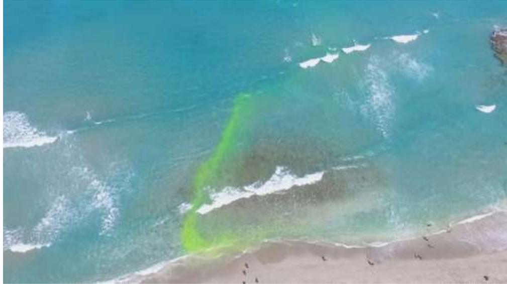
5-5. The freeze-frame from the quadcopter video shows the rip current at Ocean Reef Park as delineated by fluorescent dye; the rip is angled east-southeast as controlled by the rock outcrop.
