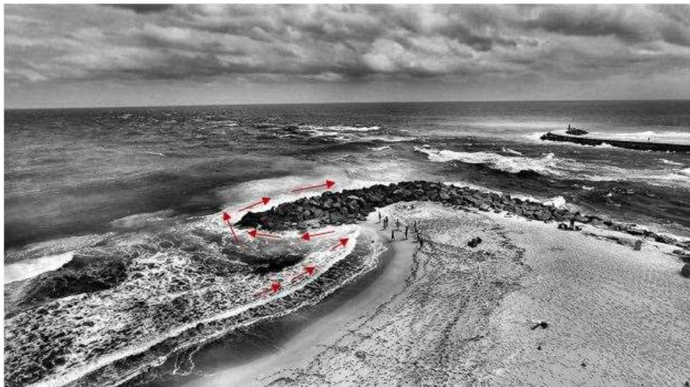
6-11. A freeze-frame from the quadcopter video shows fluorescent dye moving around the jetty and toward the strong tidal current at Haulover Inlet on April 6, 2016. The arrows represent the rip current flow path.
