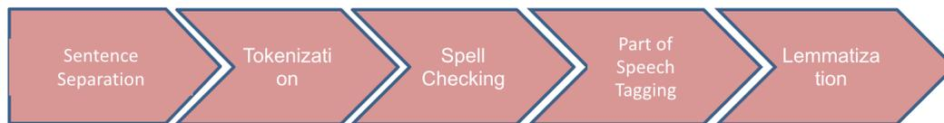
Figure 6.4: Text Preprocessing Pipeline
