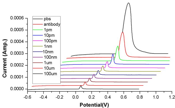
Figure 18: Different concentration of cortisol dispersed on the immunosensor and their oxidation response current.
