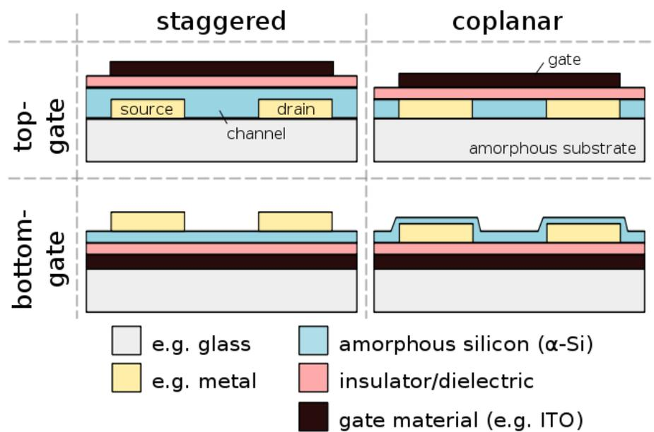
Figure 8: Different configurations of a TFT [1]
