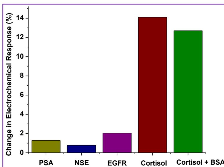
Figure 12: CV studies of EA/Anti-C<sub>ab</sub>/DTSP-SAM/IDEs immuno-electrode with respects to interferences such as PSA (100 pg/mL), NSE (100pg/mL), EGFR (100pg/mL) and BSA+Cortisol (100 pg/mL) with respect to cortisol (100 pg/mL)
