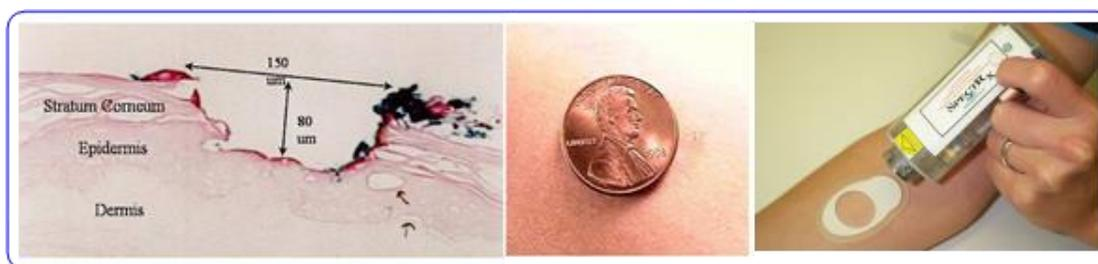
Figure 4: Left to right- Cross-section of micropore generated through laser ablation; Four pores relative to the size of a penny; Handheld laser source used to create micropores [51].
