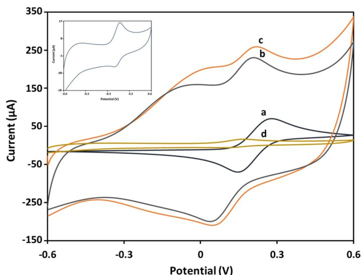
Figure 21: CV scans of 5 mM K<sub>4</sub>[Fe(CN)<sub>6</sub>]/K<sub>3</sub>[Fe(CN)<sub>6</sub>] solution at (a) bare SPCE, (b) PPy-SPCE, (c) Cortisol-PPy-SPCE and (d) MIP-PPy-SPCE; scan rate of 50 mVs<sup>-1</sup>; (Inset: Enlarged version of curve d).
