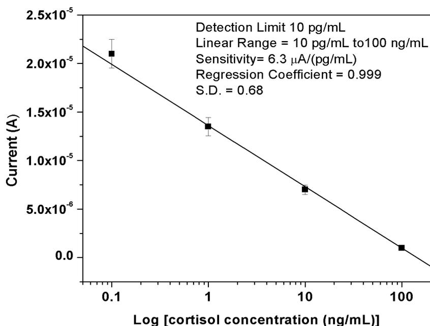
Figure 11: Calibration curve plotted between the magnitudes of current response obtained and logarithm of cortisol concentration (10 pg/mL to 100 ng/mL)
