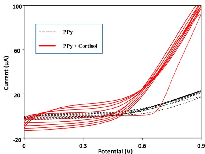
Figure 19: CV scans taken during the electropolymerization of pyrrole in the absence (dotted lines) and in the presence (solid lines) of 10 mM cortisol onto the SPCE. Scan rate: 50 mV/s.
