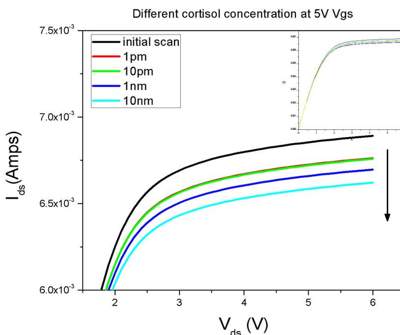
Figure 35: Output characteristics of the EGFET after adding different cortisol concentrations at a constant gate voltage of 5V
