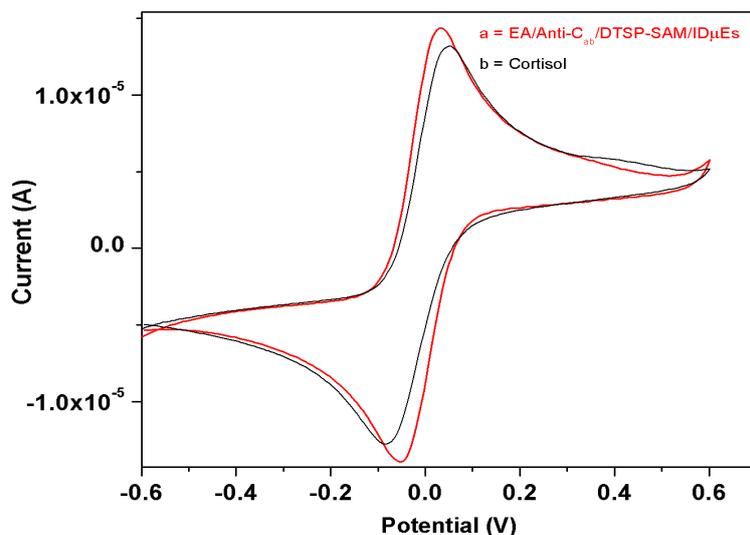
Figure 10: Electrochemical response of EA/Anti-C<sub>ab</sub>/DTSP-SAM/IDEs immunoelectrode after addition of standard cortisol solution
