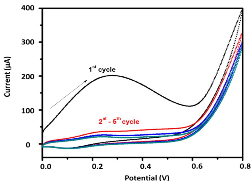
Figure 20: Recorded voltammograms during the elution of cortisol from the PPy matrix at 0.1 M PBS; scan rate of 50 mV/s.
