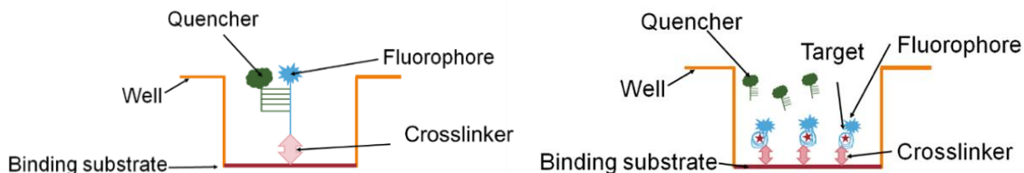
Figure 7: Depiction of immobilization of fluorophore/quencher sequence
