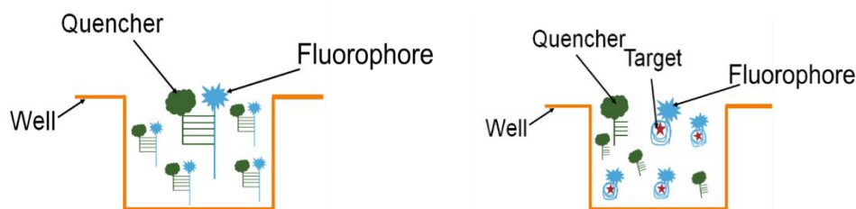
Figure 4: Proposed multiwell in solution aptamer-based assay
