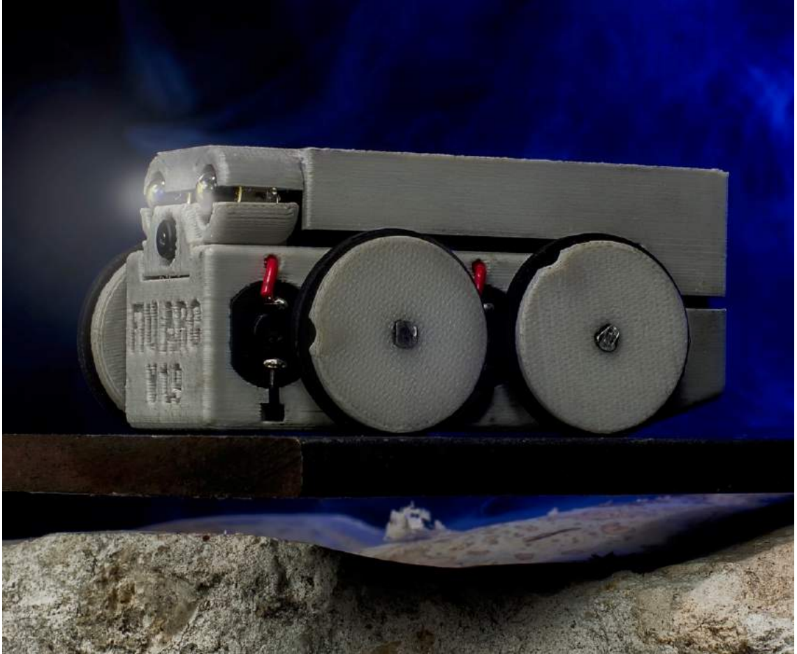
Figure 2.12: Prototype mini-rover for inspection of refractory slots.
