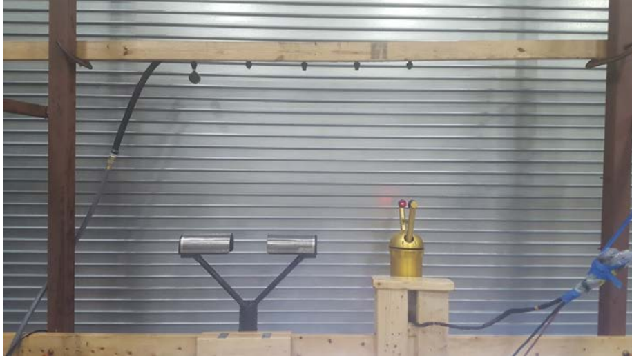
Figure 4. Droplet measurement using Parsivel and PIP for single-nozzle spray in the stagnant air
