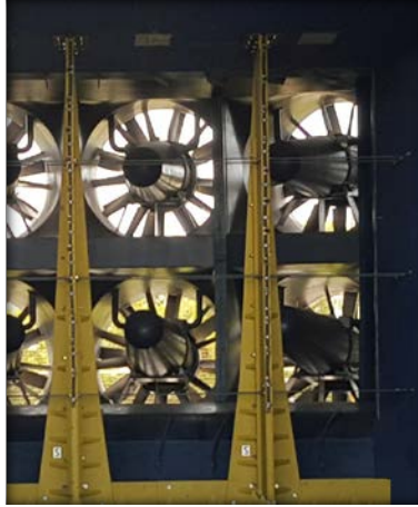
Figure 10. Vertical spires in front of the WOW EF, where the nozzles will be installed on the hoses
