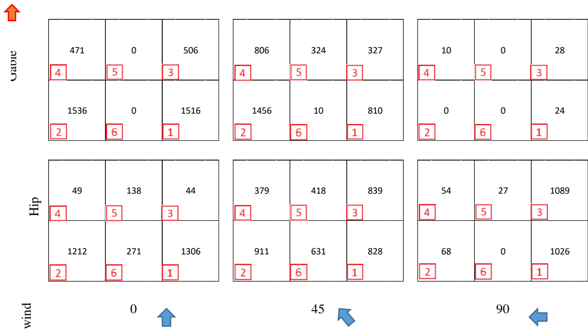
Figure 40. Attic compartments' numbering and water propagation in grams (% of total water intruded through roof openings), for the moderate damage state model
