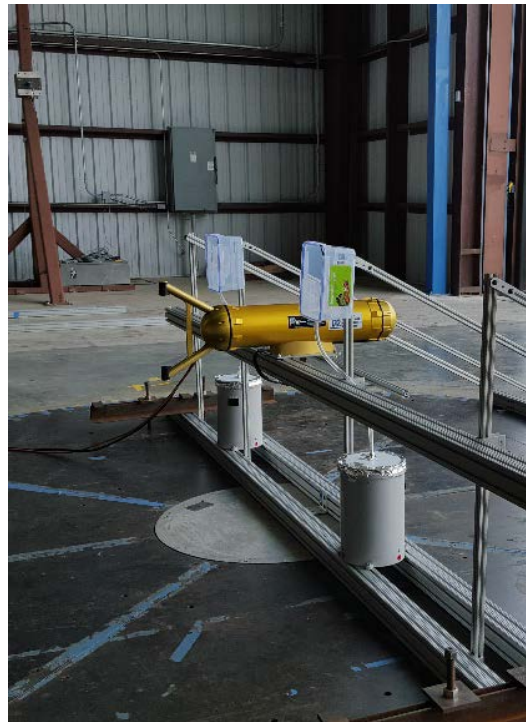
Figure 15. TB3 rain gauge connected to vertical rain-collecting bucket
