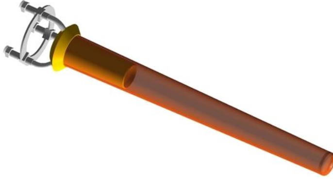
Figure 2.8: A schematic diagram of the target cell used during the g12 run period. The target cell is 40 cm long. Image source: [53]
