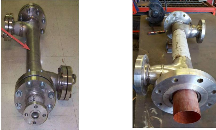
Figure 41. Pilot test module of the TMC shell and tube heat exchangers [84].
