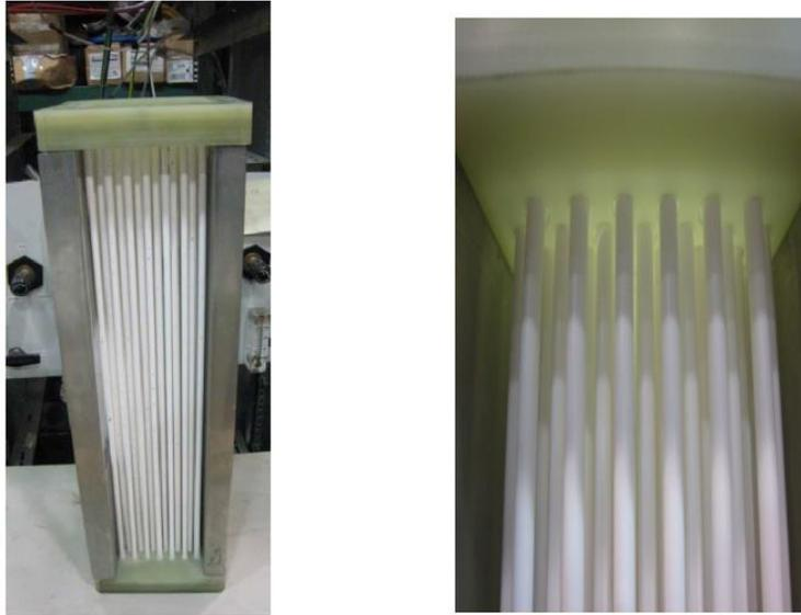
Figure 16. Lab scale TMC heat exchanger [1].
