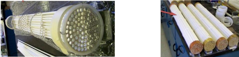
Figure 40. TMC Bundle Fabrication Layout [84].
