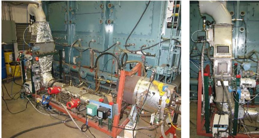
Figure 15. Experimental rig and the test section for the lab scale TMC heat exchangers.
