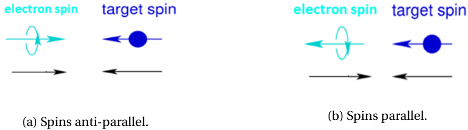
Figure 4.13: Possible longitudinal spin orientations of incident electron and target.
