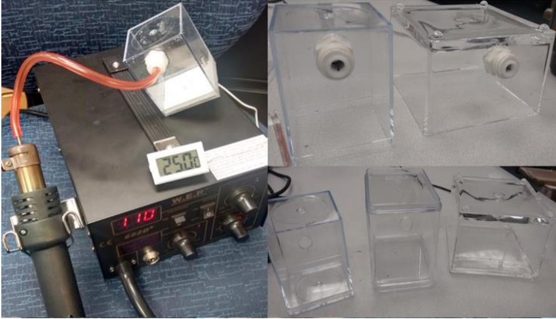
Figure 4.8. Examples of acrylic or polystyrene (plastic) boxes with drilled holes and solder reworking station external stimuli setup.
