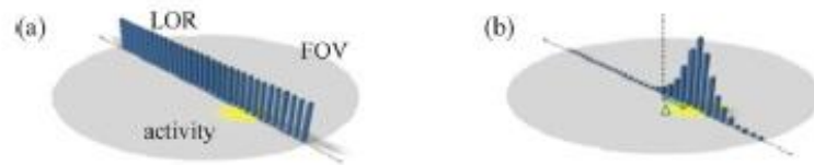
Figure 11: Equal probability assigned to all the pixels along LOR in non-TOF PET (a) and localized counts along the LOR with TOF PET (b) (47).
