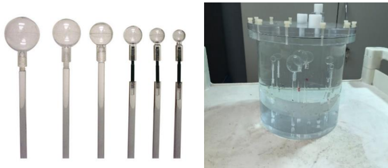
Figure 15: Different size hollow spheres (left) and Jaszczak phantom with spherical inserts (right).
