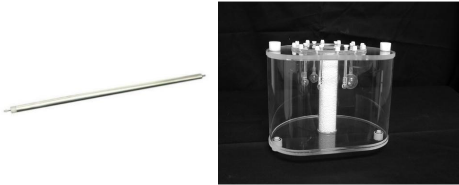
Figure 28: (left) Rod phantom and (right) IEC body phantom used in calibration factor study (68).
