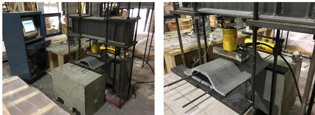
Figure 3-25 Shear specimen SC-S under testing load
