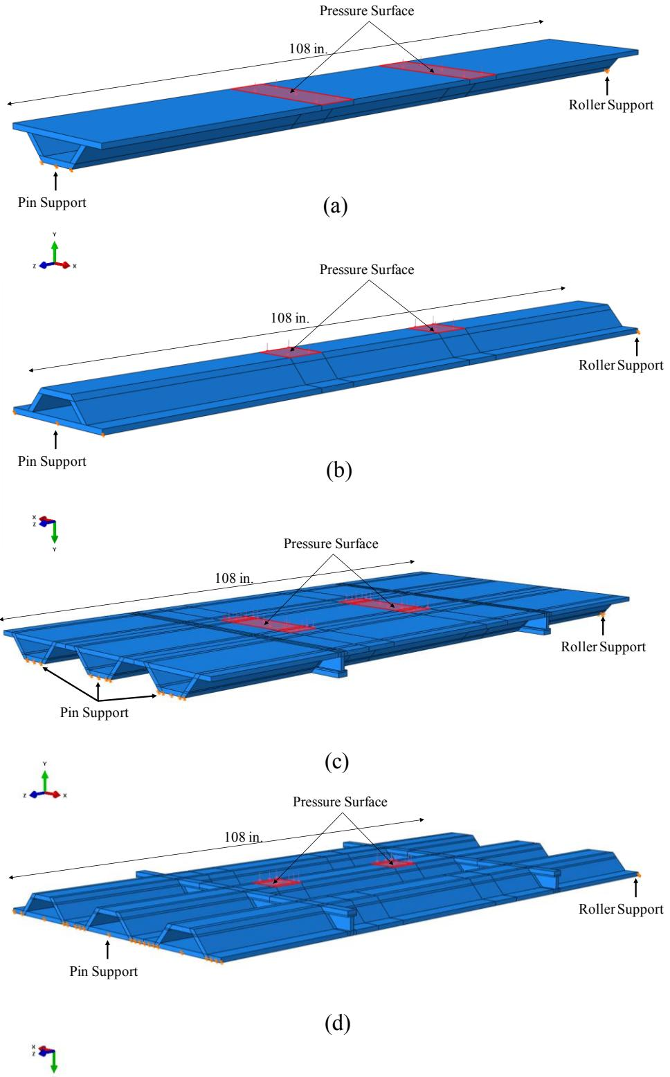
Figure 4-1 Finite Element model of laboratory specimens; (a) SC-P; (b) SC-N; (c) MC-P; (d) MC-N
