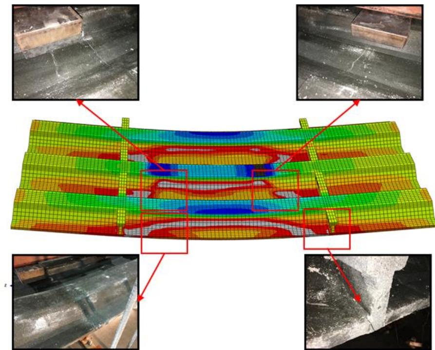
Figure 4-7 Stress distribution on the deflected shape and failure mode of specimen MC-N
