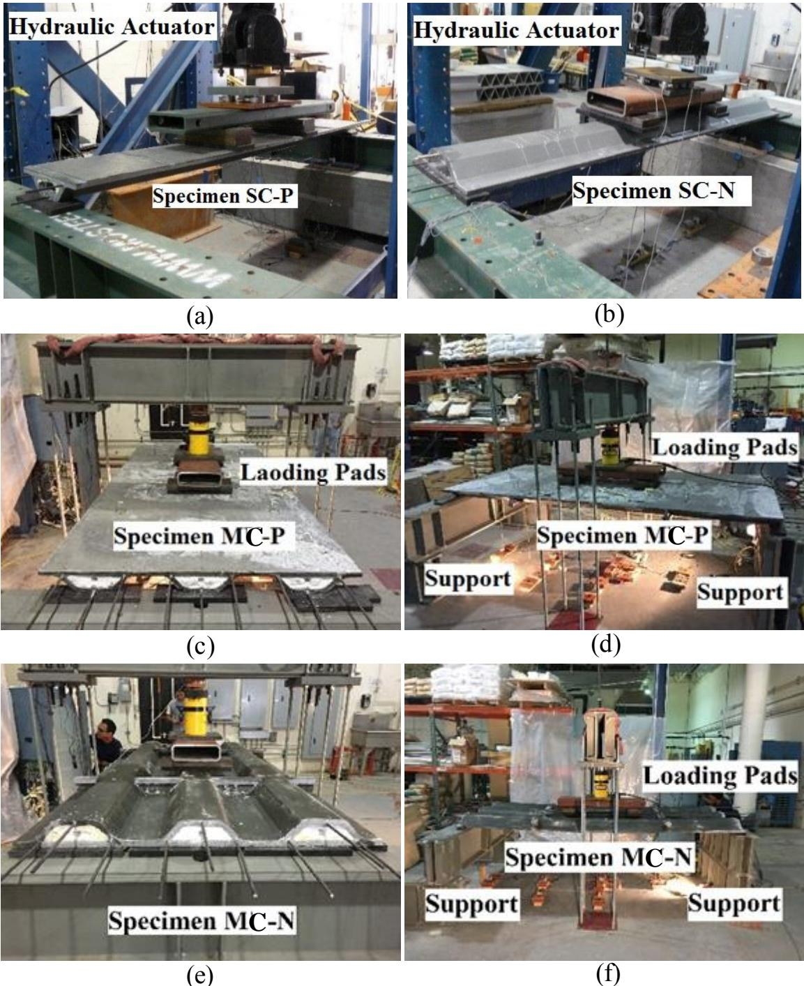
Figure 3-11 Flexure test setup: (a) Specimen SC-P; (b) Specimen SC-N; (c and d) Specimen MC-P; (e and f) Specimen MC-N
