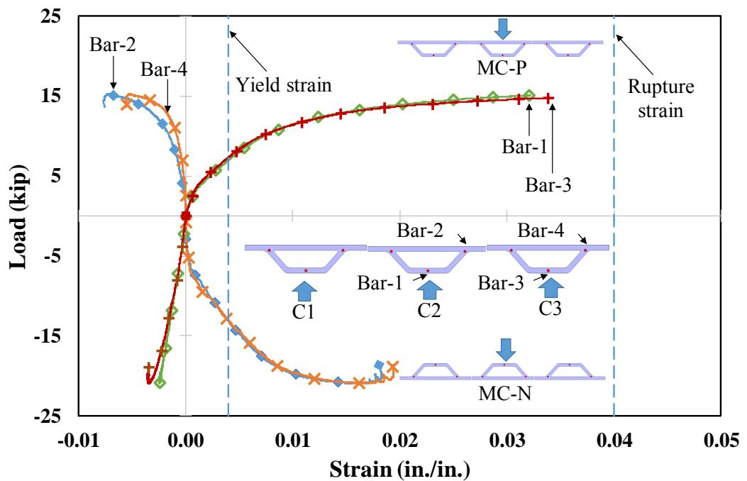
Figure 3-19 Load-Strain responses of HSS reinforcement of Multi-cell specimens
