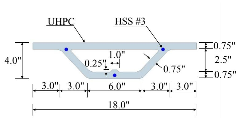
Figure 2-8 Geometric details of the engineered box-cell section
