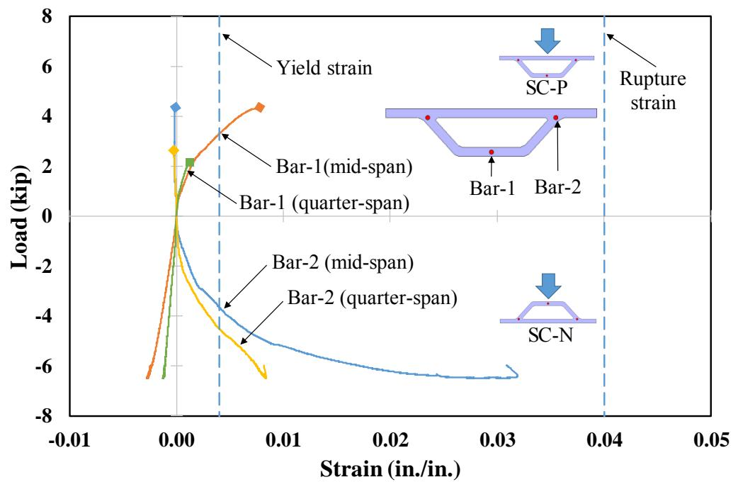
Figure 3-18 Load-Strain responses of HSS reinforcement of Single-cell specimens
