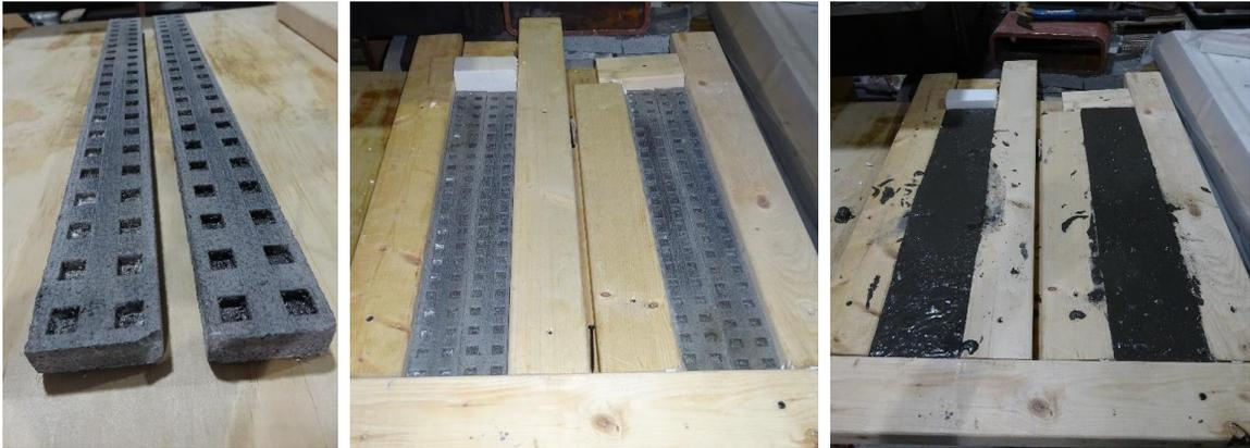
Figure 5-3 Group 1 connection specimen preparation, FC-P and FC-N specimens
