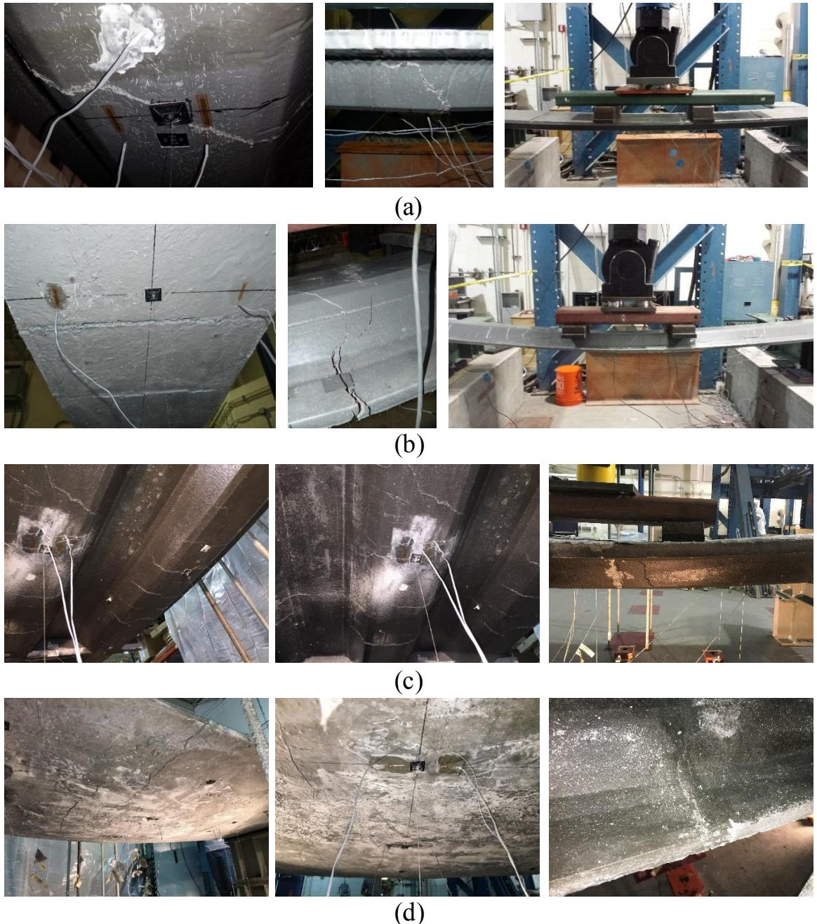
Figure 3-15 Flexural test modes of failure; (a) SC-P; (b) SC-N; (c) MC-P; (d) MC-N
