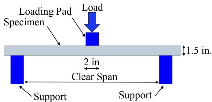
Figure 5-5 Test setup for flange connection
