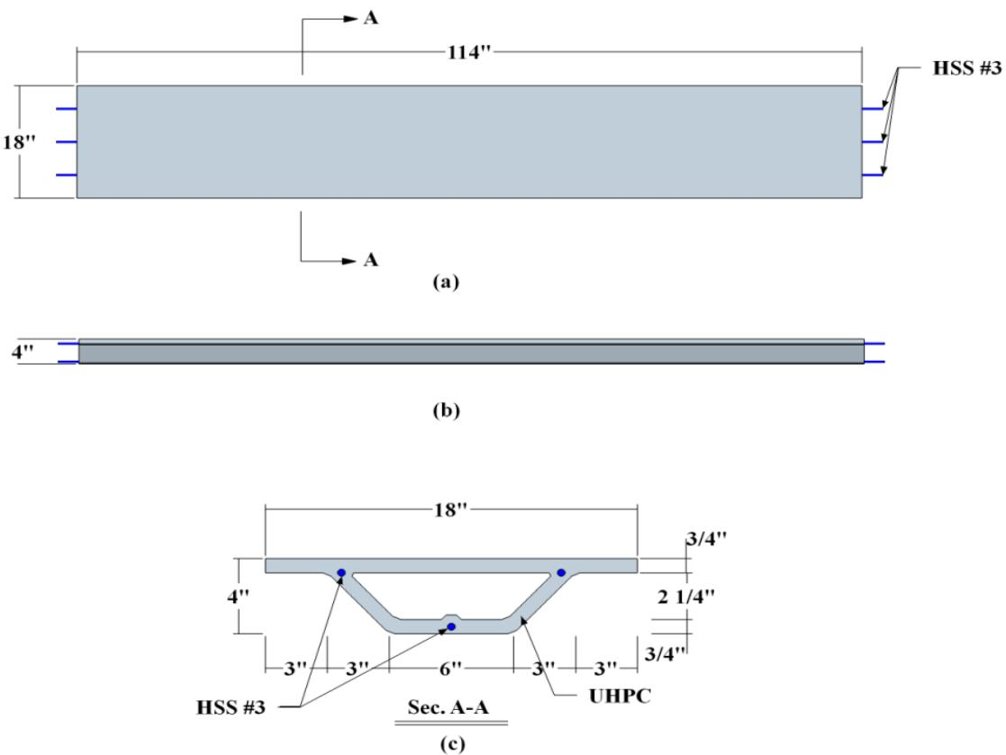
Figure 3-1 Schematic of Single-cell Specimen: (a) Plane view; (b) Side view; (c) Cross-section
