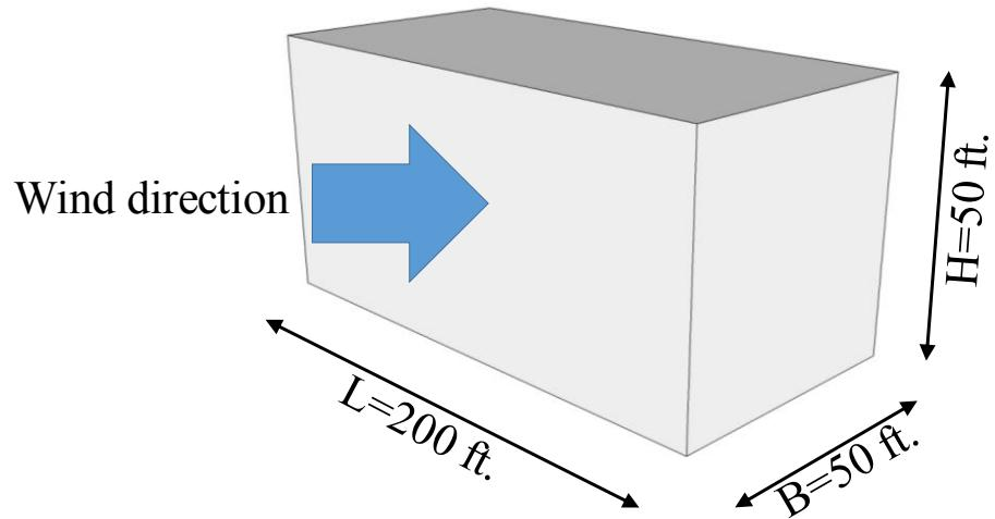
Figure 2-1 The case study building dimensions and wind configuration
