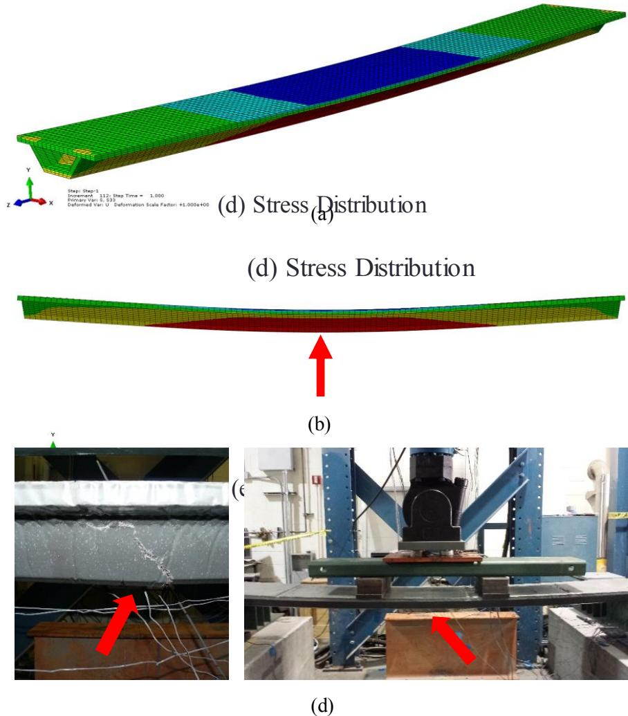
Figure 4-4 Deflected shape and failure mode of specimen SC-P: (a) Stress distribution, top view: (b) Stress distribution, side view (c) Failure mode in experimental test
