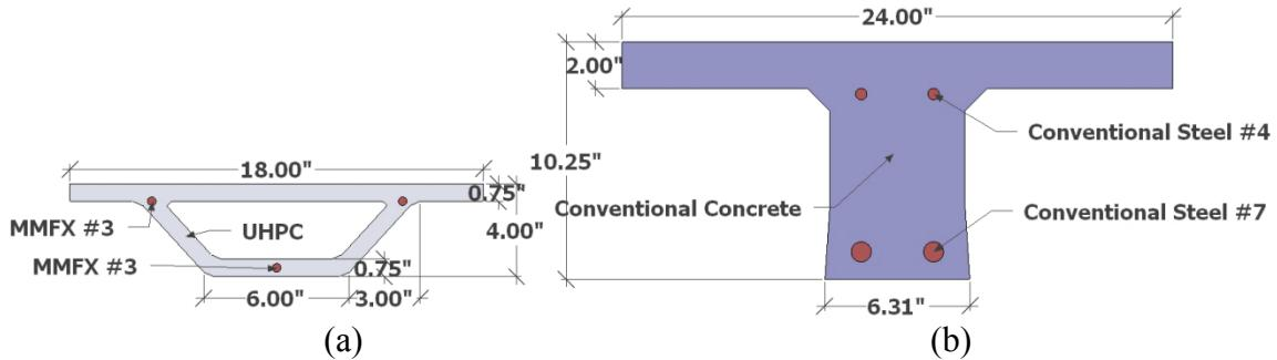
Figure 6-1 Cross section of the new roof system compared to Lite-Deck deck system
