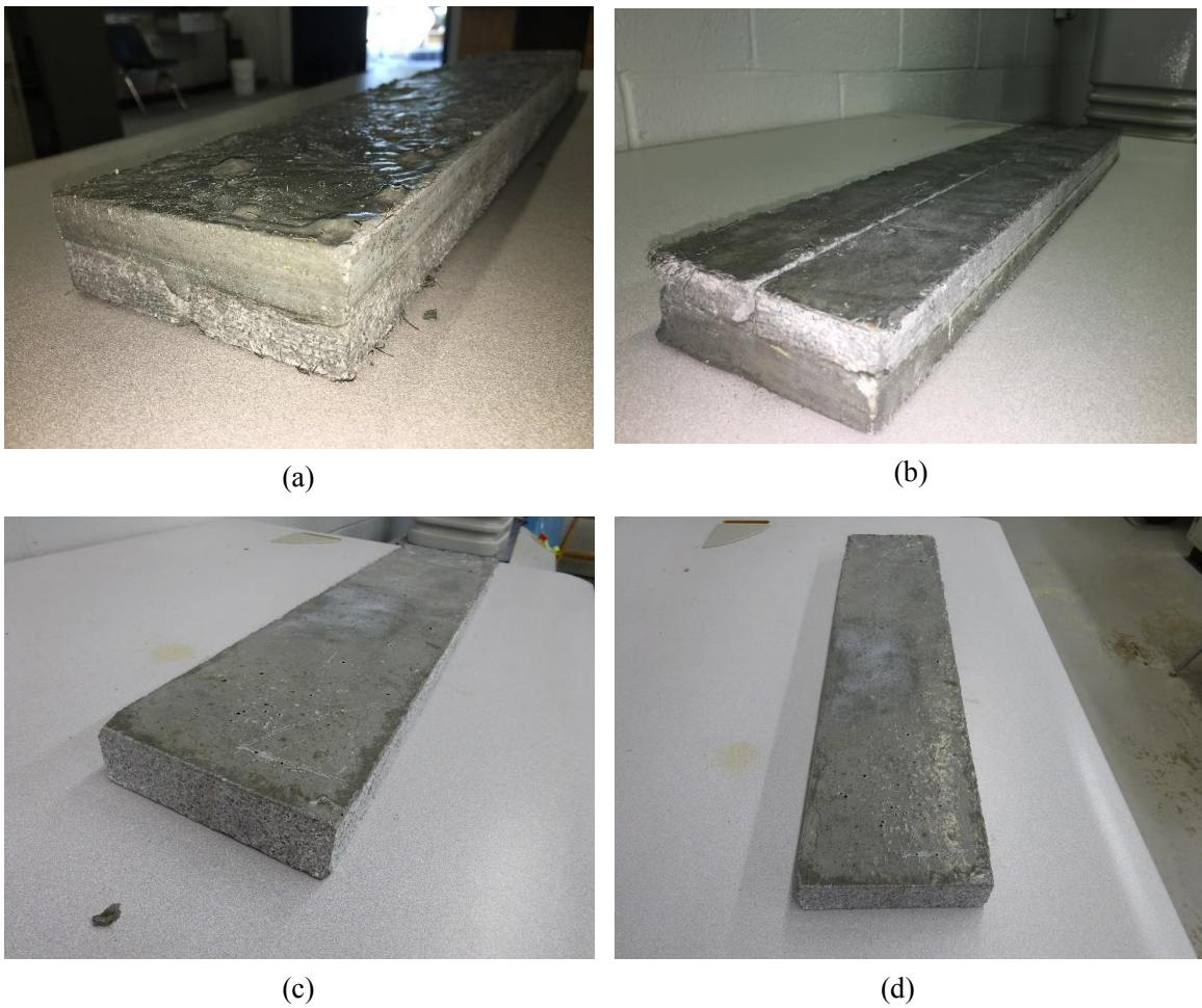
Figure 5-4 Simplified flange connection samples: (a) FC-P Specimen; (b) FC-N specimen; (c) SOLID-1 specimen; (d) SOLID-2 specimen
