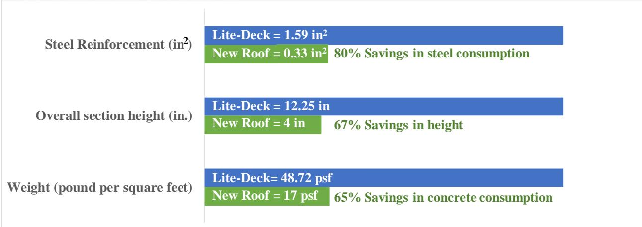
Figure 6-2 The new roof system improvement compared to Lite-Deck
