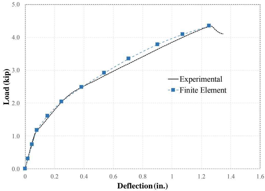
Figure 4-8 Load-Deflection response of SC-P at mid-span
