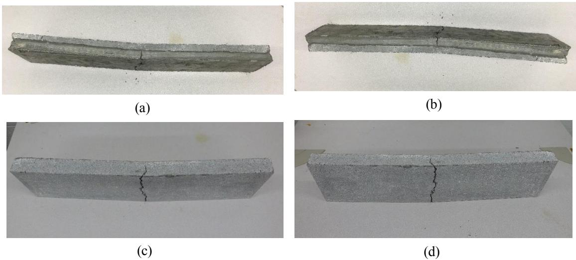
Figure 5-9 Failure mode of flange connection samples: (a) FC-P specimen; (b) FC-N specimen; (c) SOLID-1 specimen; (d) SOLID-2 specimen
