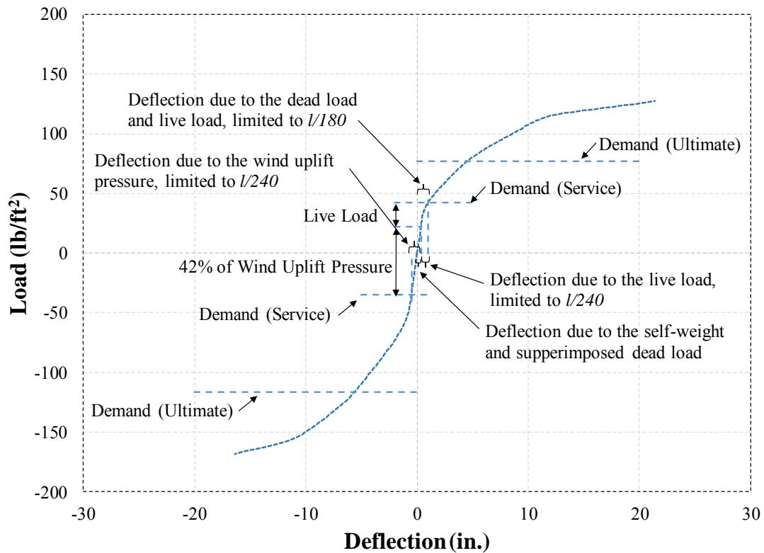
Figure 4-14 Load-Deflection response of proposed roof panel for 20 ft. span with nonplaster ceiling, resulted from finite element models
