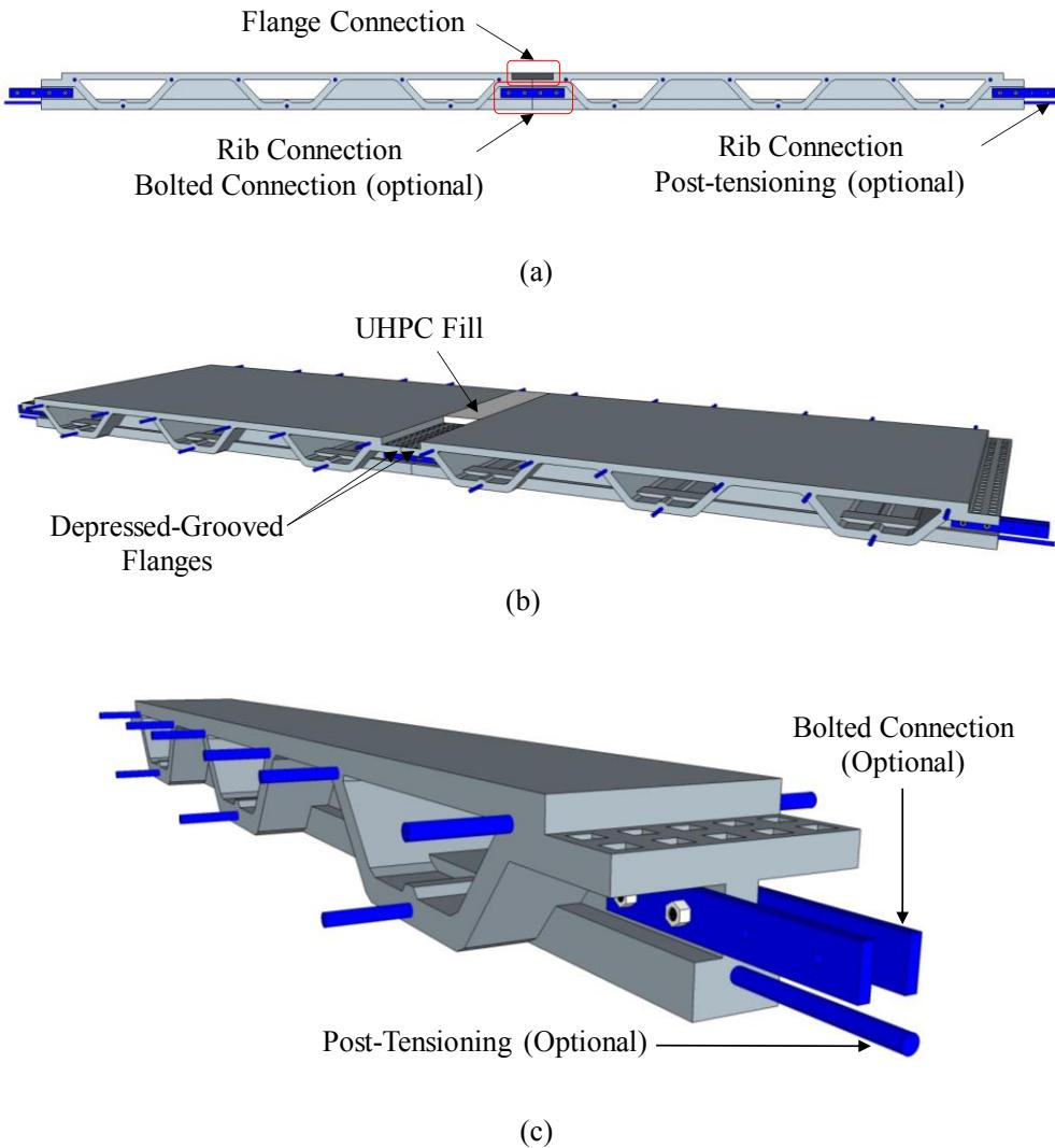
Figure 5-1 Panel-to-Panel connection and its components: (a) Components of Panel-to-Panel connection; (b) Flange connection; (c) Rib connection
