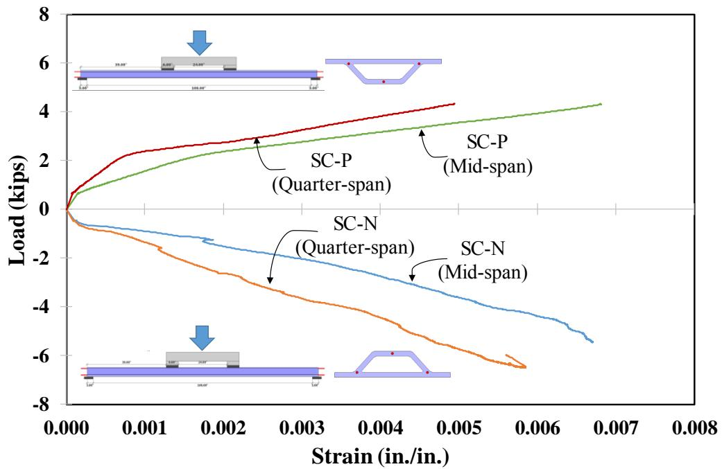
Figure 3-20 Load-Tensile strain responses of UHPC in Single-cell specimens
