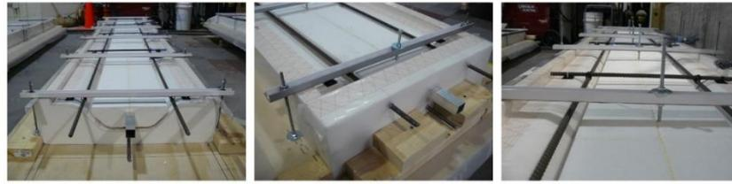
Figure 3-3 Formwork made of Styrofoam for single-cell specimens
