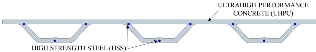
Figure 2-5 The initial cross-sectional shape considered for the development of the new roof system
