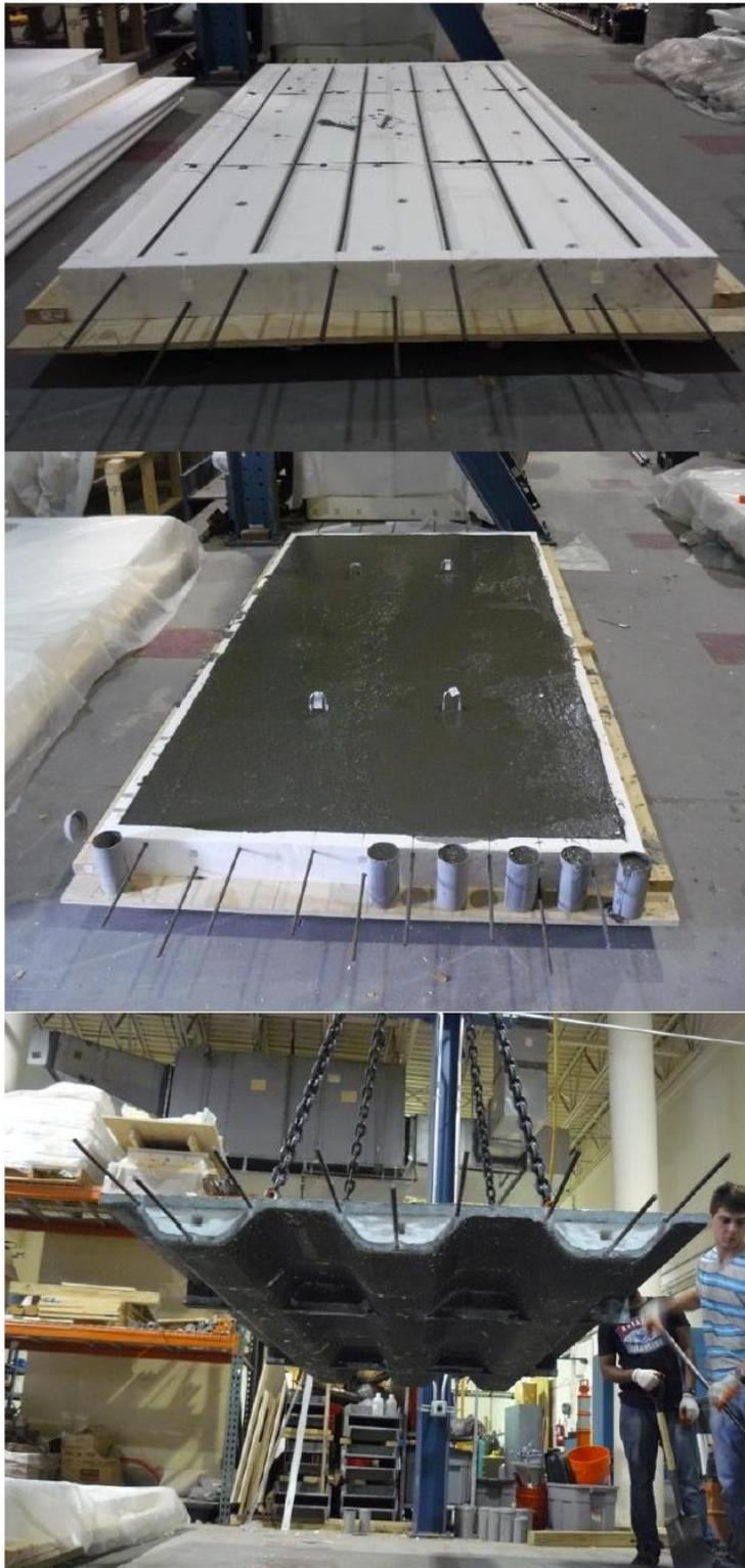
Figure 3-6 Multi-cell specimens preparation
