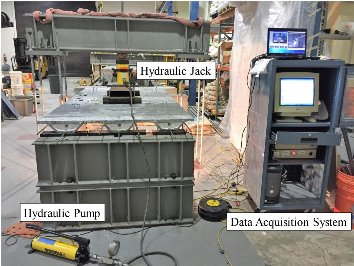
Figure 3-14 Loading system utilized for testing of Multi-cell specimens
