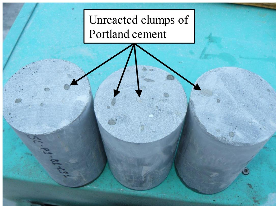
Figure 3-10 Minute unreacted clumps of Portland cement in the hardened UHPC matrix of SC-P specimen, due to the lack of experienced construction personnel and selection of improper mixing equipment
