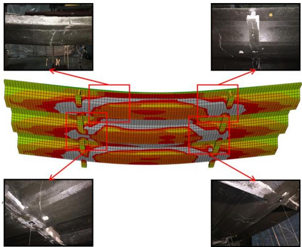
Figure 4-6 Stress distribution on the deflected shape and failure mode of specimen MC-P
