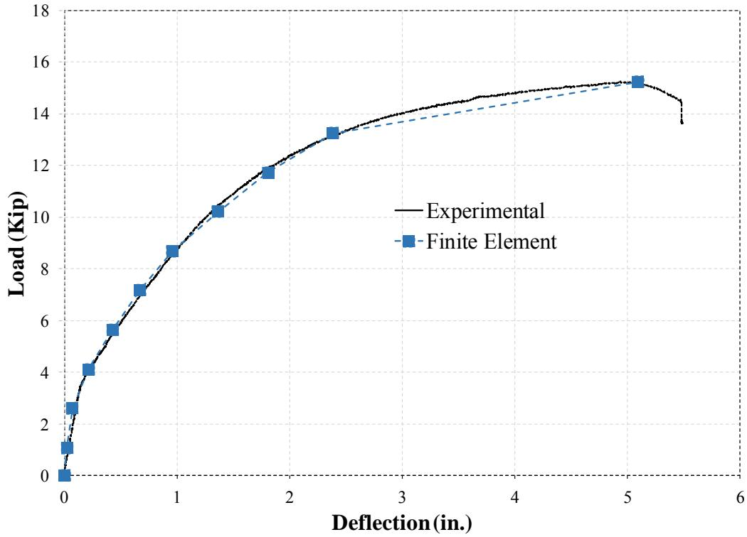
Figure 4-10 Load-Deflection response of MC-P at mid-span of middle unit (C2)
