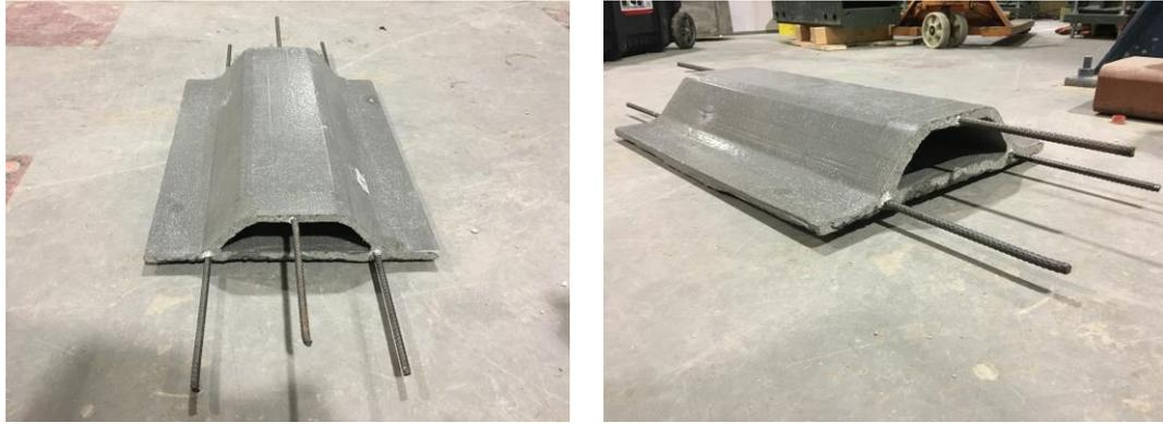
Figure 3-23 Shear specimen (SC-S)
