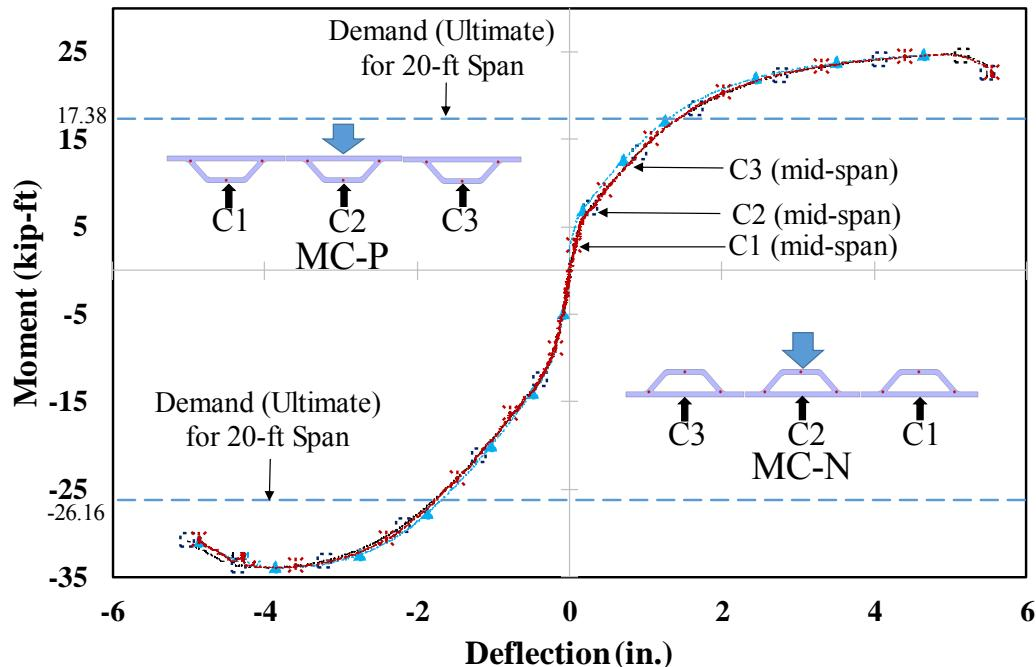
Figure 3-21 Moment-Deflection responses at mid-span of Multi-cell specimens
