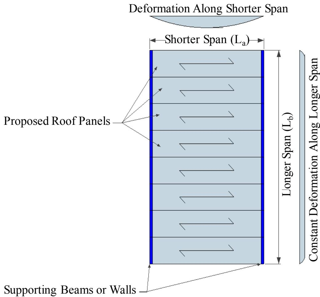
Figure 2-7 Structural action of the proposed roof system
