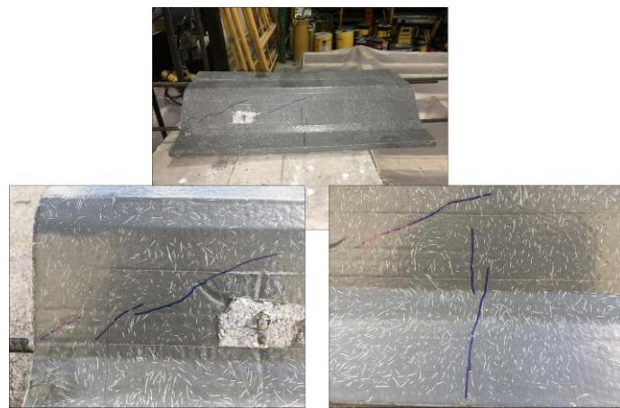
Figure 3-26 Shear test mode of failure and crack patterns, specimen SC-S
