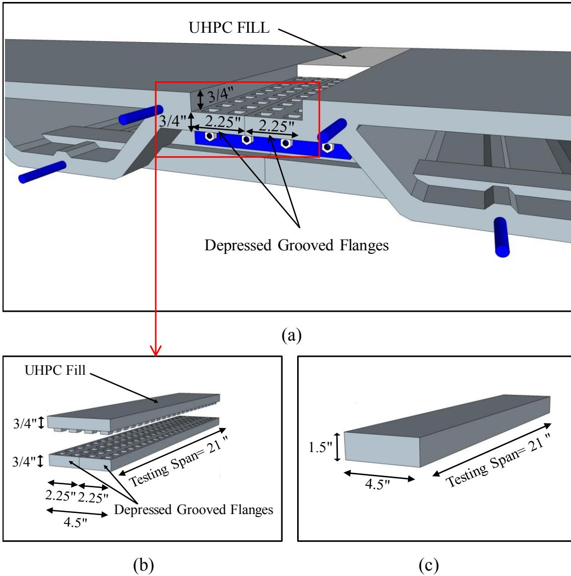
Figure 5-2 Details of flange connection as the Panel-to-Panel connection compartment; (a) Geometric details; (b) Geometric details of Group 1 connection specimens; (c) Geometric details of Group 2 specimens
