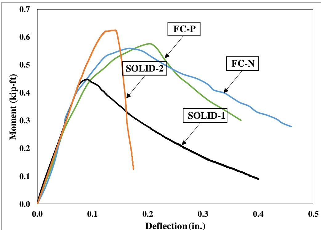
Figure 5-10 Moment-Deflection response of flange connections (panel-to-panel specimen connections)
