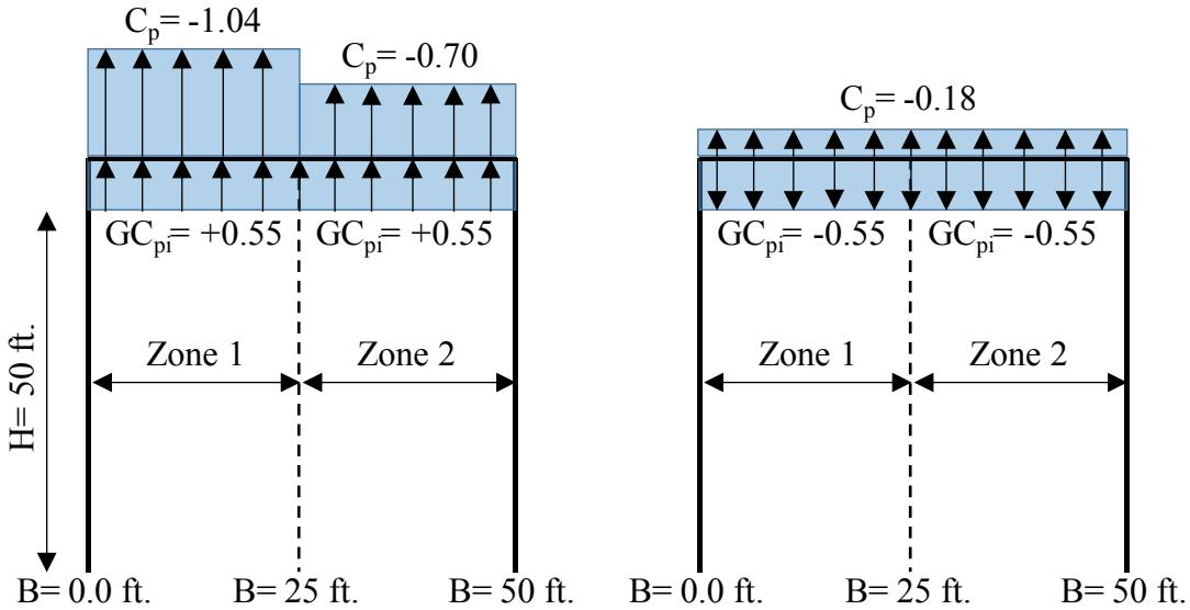
Figure 2-2 Internal and external pressure coefficients on the flat roof of the building
