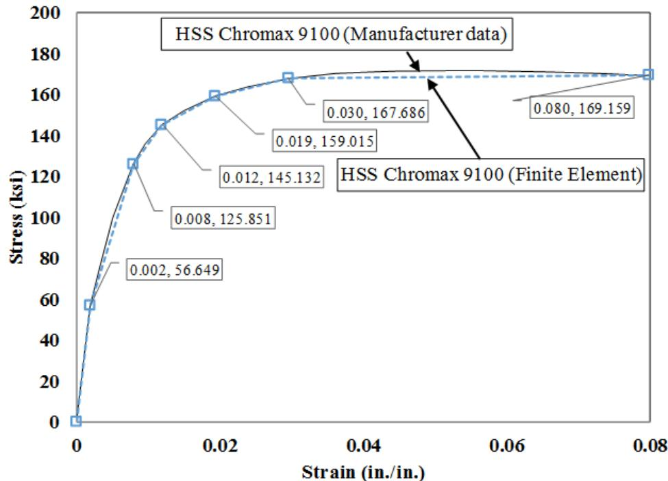
Figure 4-3 Uniaxial stress-strain responses of HSS ChromaxX 9100 (Grade 100) and equivalent responses used for FE modeling
