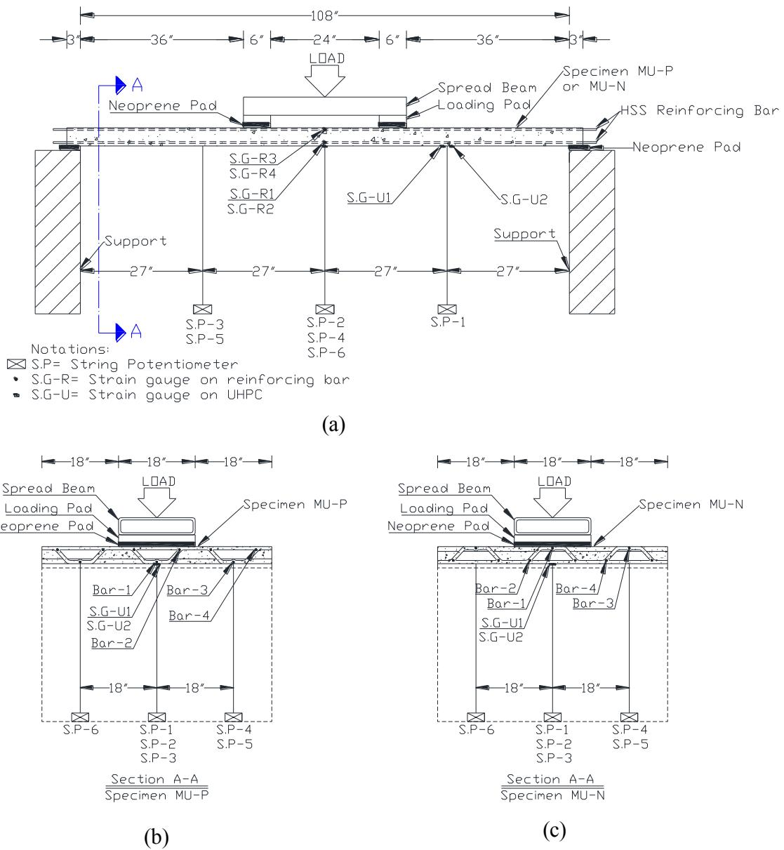
Figure 3-13 Test setup and instrumentation details of Multi-cell specimens: (a) Side view; (b) Specimen MC-P; (c) Specimen MC-N
