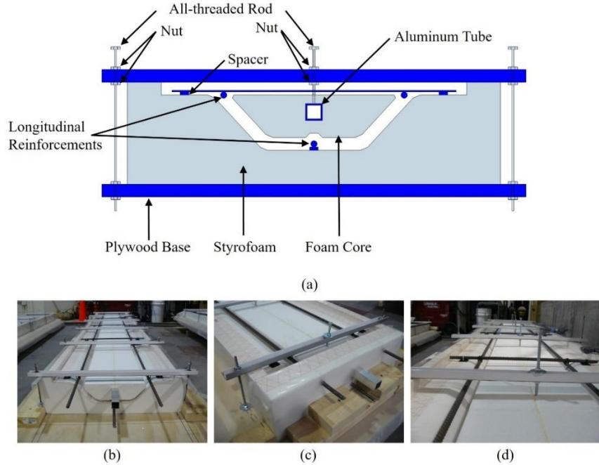
Figure 3-3 Formwork made of Styrofoam for single-cell specimens
