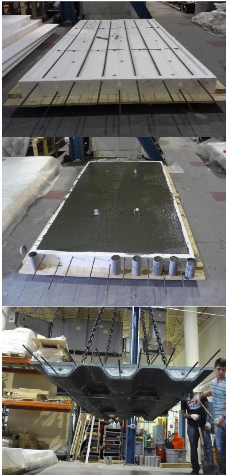
Figure 3-6 Multi-cell specimens preparation
