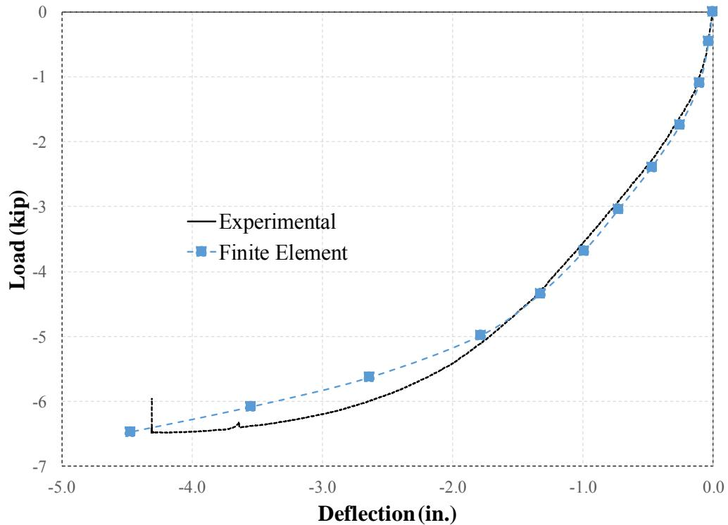
Figure 4-9 Load-Deflection response of SC-N at mid-span
