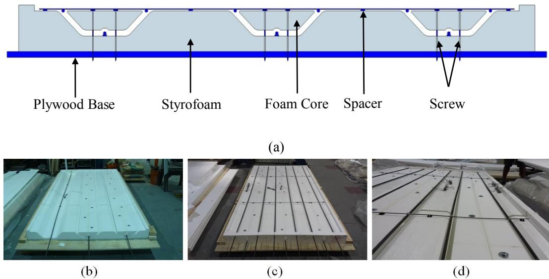
Figure 3-4 Formwork made of Styrofoam for Multi-cell panel specimens
