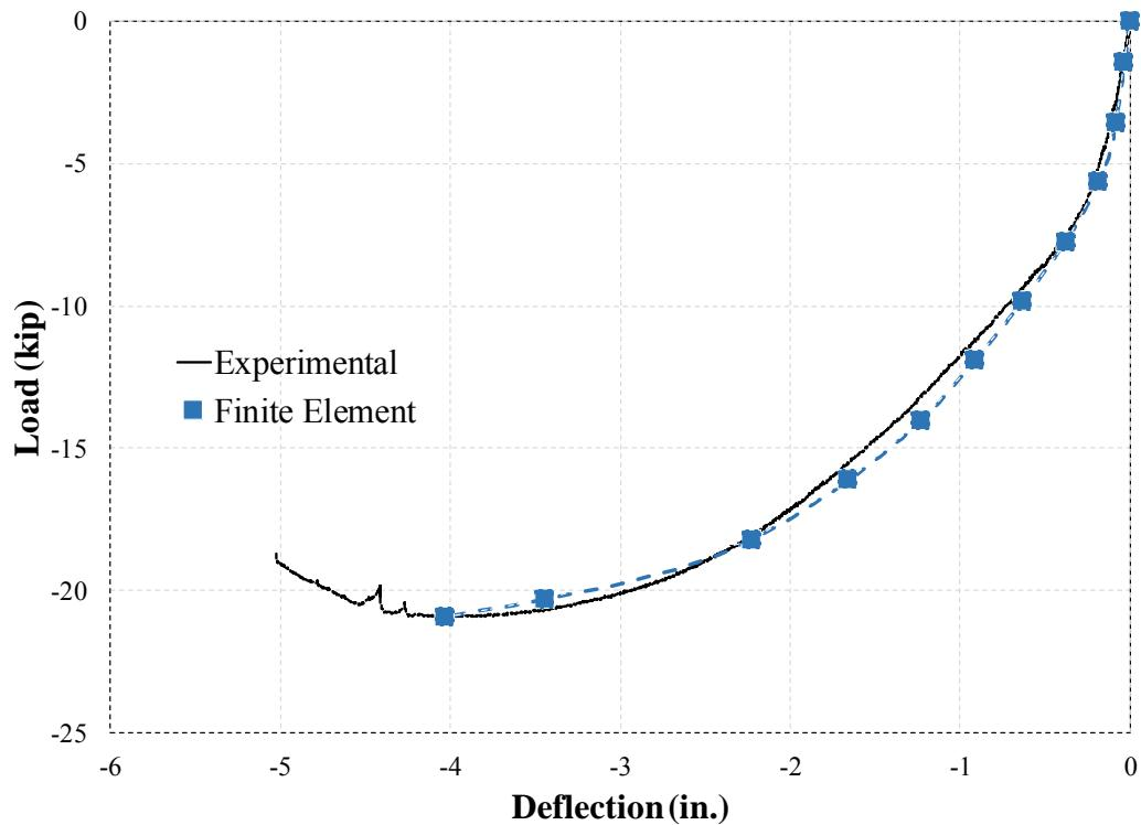
Figure 4-11 Load-Deflection response of MC-N at mid-span of middle unit (C2)
