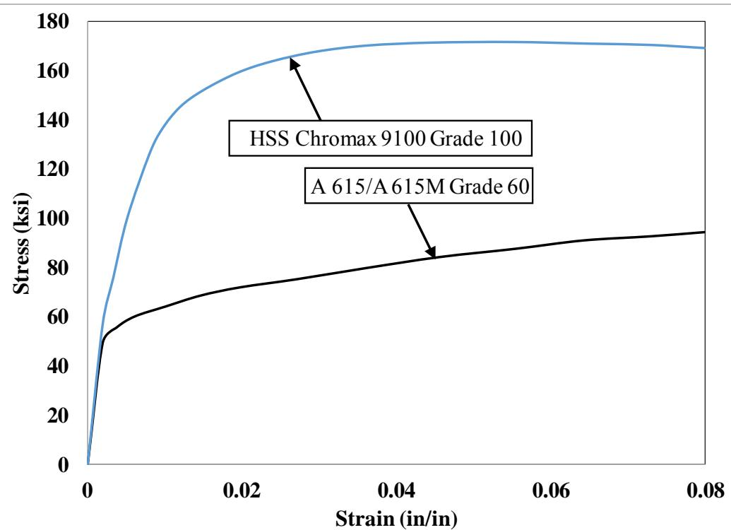
Figure 2-3 Stress-Strain responses of high strength steel (HSS), ChromaX 9100, and steel grade 60
