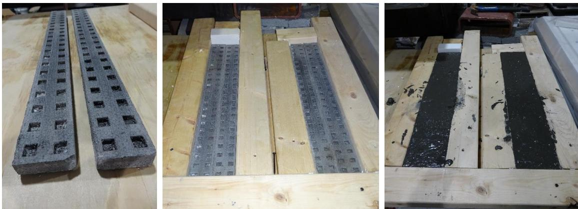
Figure 5-3 Group 1 connection specimen preparation, FC-P and FC-N specimens
