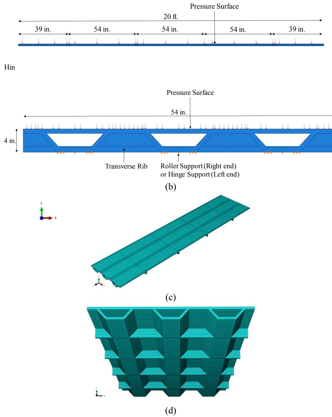
Figure 4-12 Finite Element model of 20-foot multi-cell roof panel: (a) Side view; (b) Cross section; (c) Top view; (d) Bottom view
