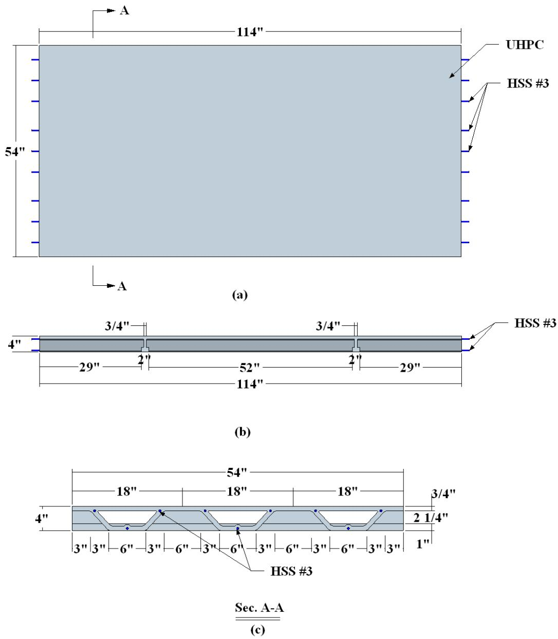
Figure 3-2 Schematics of Multi-cell Specimen: (a) Plan view; (b) Side view; (c) Cross-section
