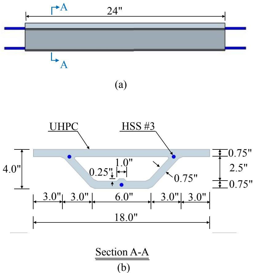
Figure 3-22 Geometric details of shear specimen (SC-S)
