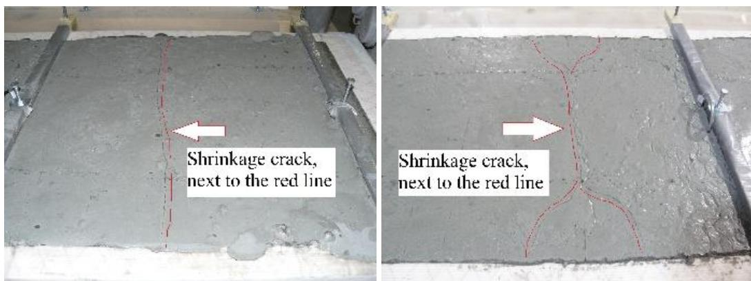
Figure 3-9 Lateral shrinkage cracks on the top flange of SC-P specimen due to the high w/c ratio in the UHPC mix
