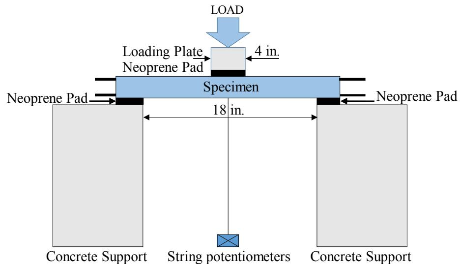
Figure 3-24 Test setup and instrumentation with shear specimen SC-S
