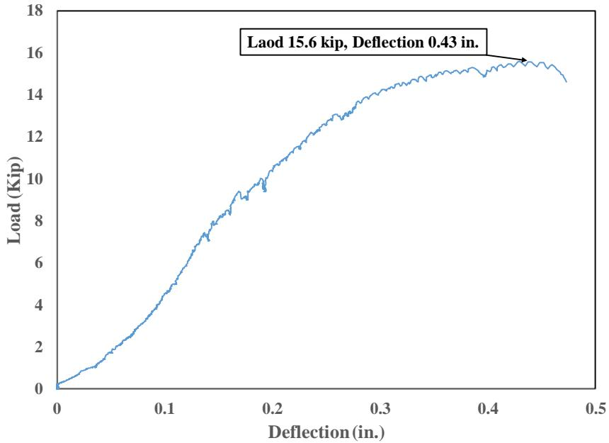
Figure 3-27 Load-Deflection response of shear test
