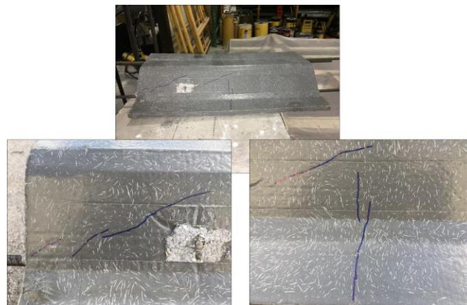
Figure 3-26 Shear test mode of failure and crack patterns, specimen SC-S
