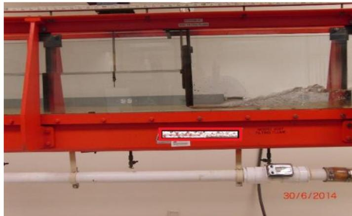
Figure 5.1.4. (a): Hydraulic jump after the gate ( $St = 0$ )
