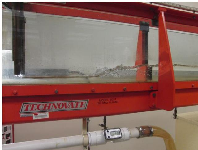
Figure 5.2.1. (a): Supercritical flow after the gate
