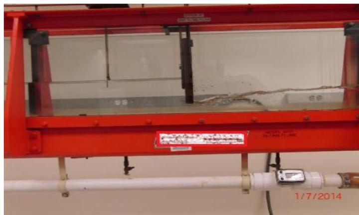
Figure 4.1. (c): Submerged hydraulic jump after the gate ( $St = 0.2$ )
