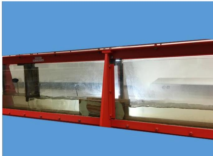
Figure 5.4.2. (b): Stable flow in the presence of a gate with contractions
