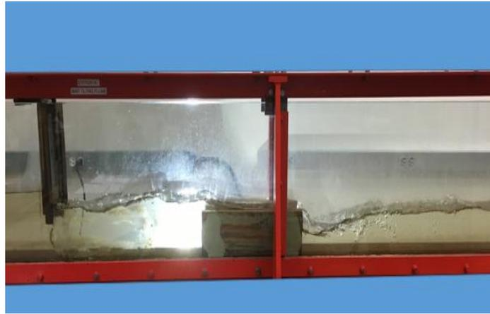
Figure 5.4.2. (a): Flow fluctuations in the presence of a gate with contractions
