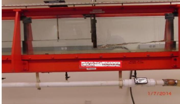
Figure 4.1. (d): Weak submerged hydraulic jump after the gate ( $St = 0.4$ )
