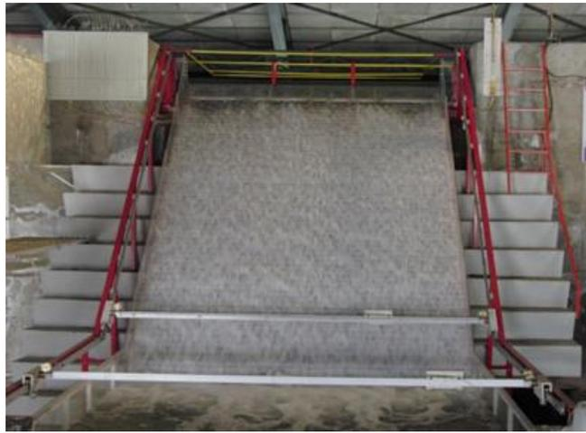
Figure 5.6.2. (a): Stepped spillway physical model, the Water Research Institute
