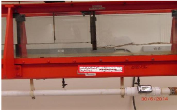
Figure 4.1. (h): Weak wave after the gate ( $St = 0.8$ )
