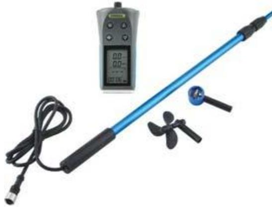
Figure 4.16: Digital velocity meter (globalindustrial.com)
