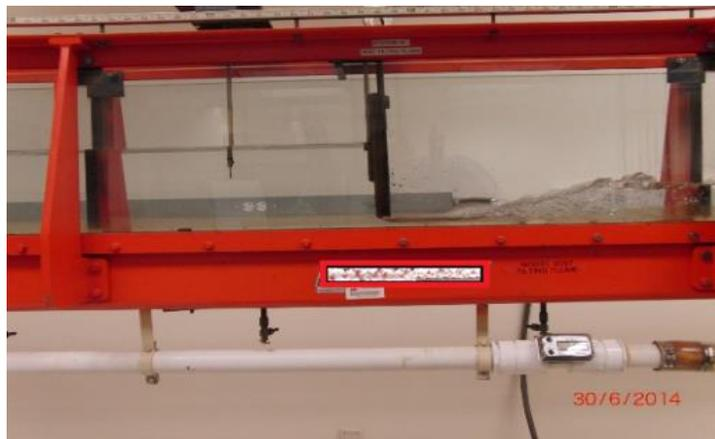
Figure 4.1. (b): Hydraulic jump after the gate ( $St = 0$ )
