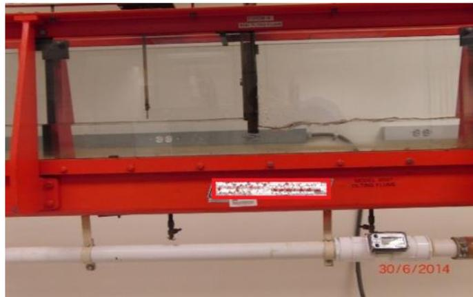
Figure 4.1. (i): Very weak wave after the gate ( $St = 0.9$ )
