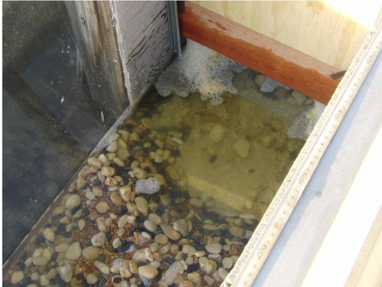
Figure 5.2.6 (a): Sediment transport after the gate
