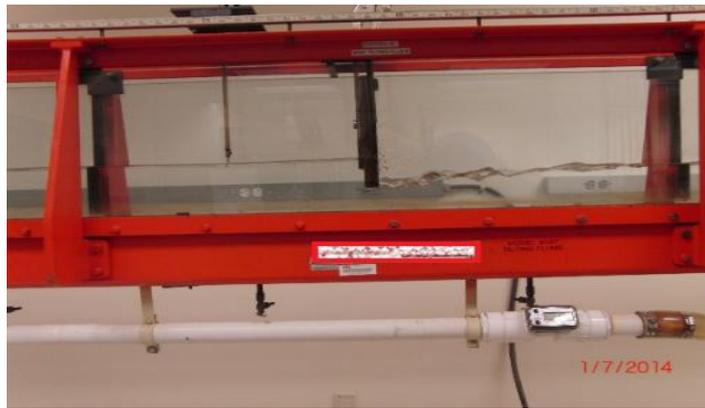
Figure 4.1. (e): Very weak submerged hydraulic jump after the gate ( $St = 0.5$ )
