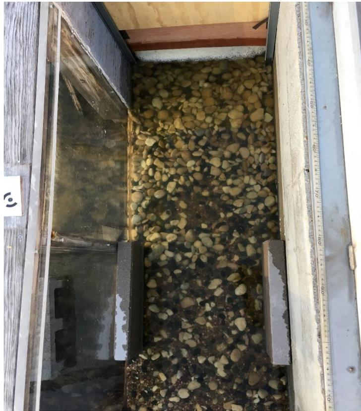
Figure 4.14. (b): Gate with contraction, plan view
