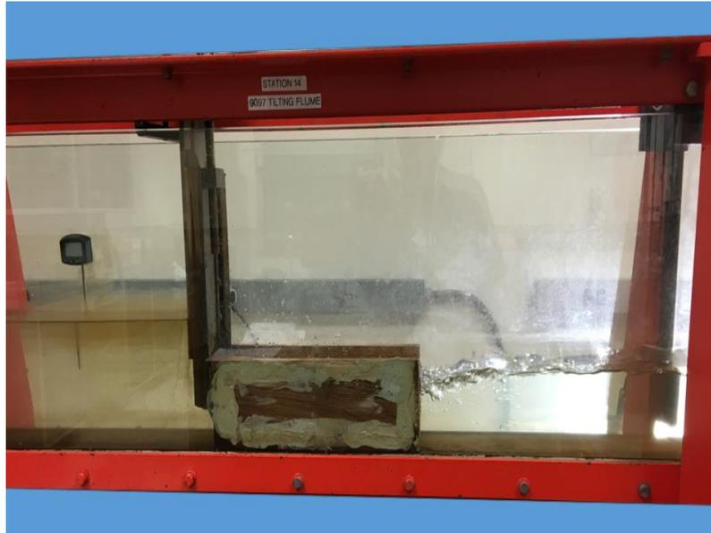
Figure 5.3.2 (a): Flow fluctuations after a gate with expansion
