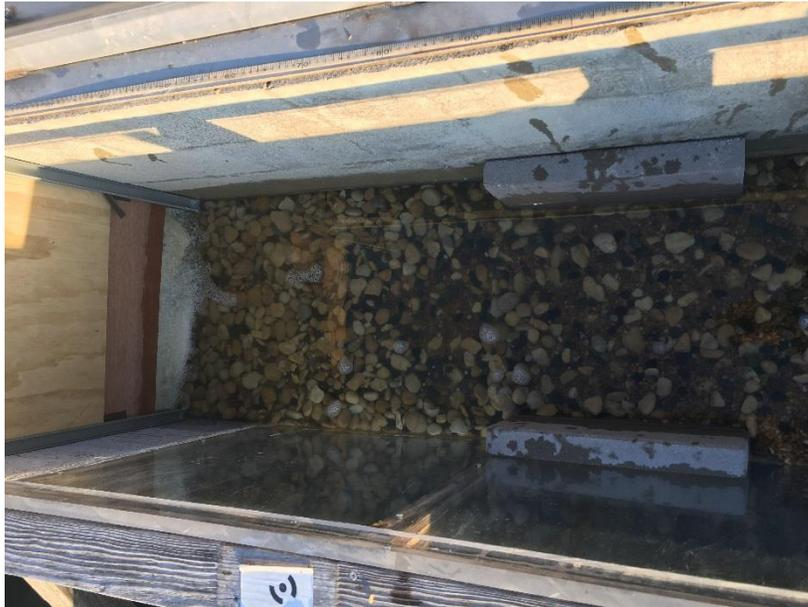
Figure 5.4.8 (a): Sediment transport in the presence of a gate with contractions
