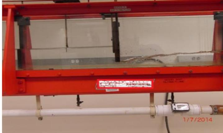
Figure 5.1.4. (b): Submerged hydraulic hump after the gate ( $St = 0.2$ )
