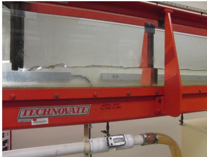
Figure 5.2.1. (b): Subcritical flow after the gate
