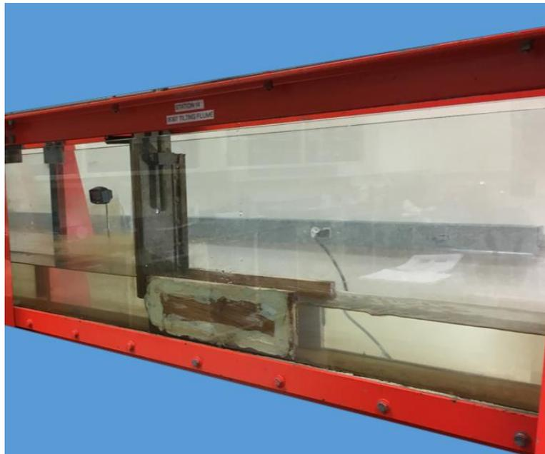
Figure 5.3.2(b): Stable flow after a gate with expansion
