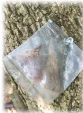
Figure 2. The controlled odor mimic permeation system with infected avocado wood sealed inside
