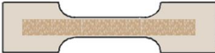
Fig. 3.3. Schematic of GrF-epoxy mold casted composite.
