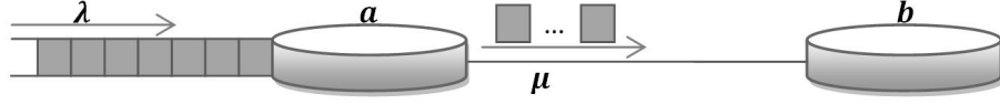
Figure A.4: The schematic view of a link and two routers. Data packets enter router a with the average rate \lambda and exits with the average rate \mu .
