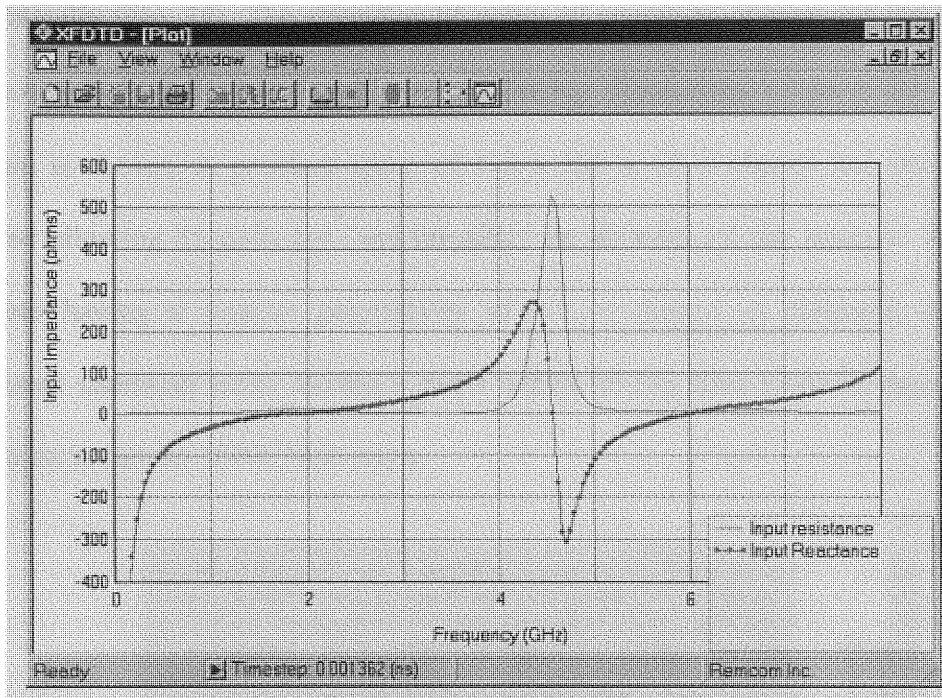
Fig. 17. Frequency Vs. input impedance for diamond dipole antenna.
