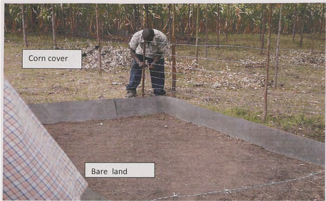
Figure 3.5 Runoff plots on bare land and corn covered in the Amala upstream
