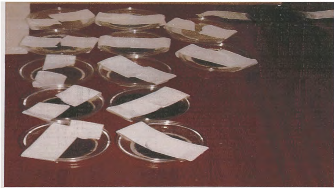
Figure 3.6 Sediment sampling method using petri dish to determine the sediment load for every rainfall event
