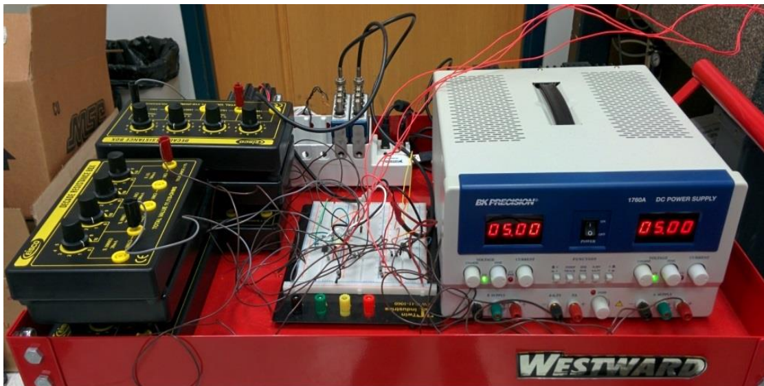
Figure 4.24 Wheatstone bridge setup for load sensing.
