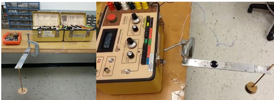
Figure 3.5 Strain sensor test setup.
