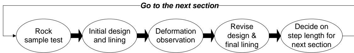
Figure 4-4 Processes of the Tunneling Project
