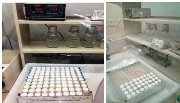
Figure 8. Sacrificial vials inside the anaerobic chamber through sampling period.
