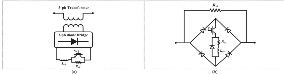
Figure 2.13: Fault current limiter topology. (a) Bridge-type FCL (BFCL). (b) Modified configuration of BFCL.
