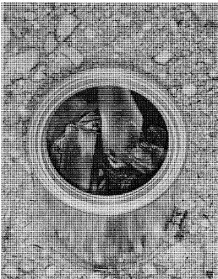
Figure 6: Mixed matrix sample burning in a paint can
